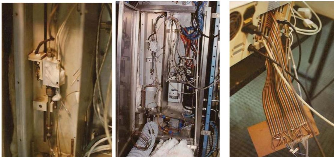
Figure 1: Partly melted heating blok at center of picture. Figure 2: The inside of the GC after the incident. Figure 3: Wiring on back of IBM AT PC with connections to GC.
