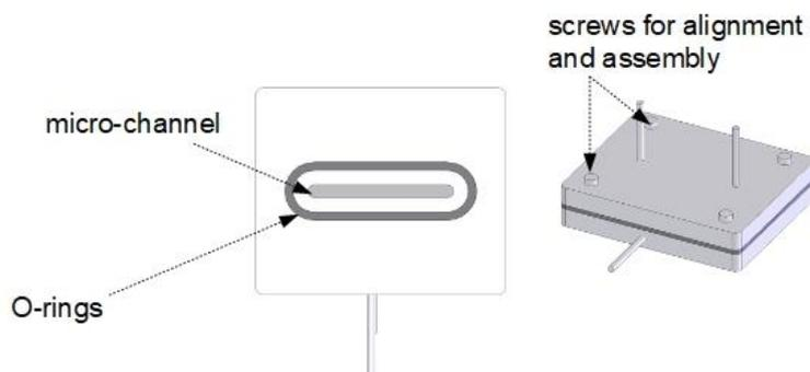
Figure 2: Basic configuration for a flat, horizontal microfluidic membrane filtration unit
