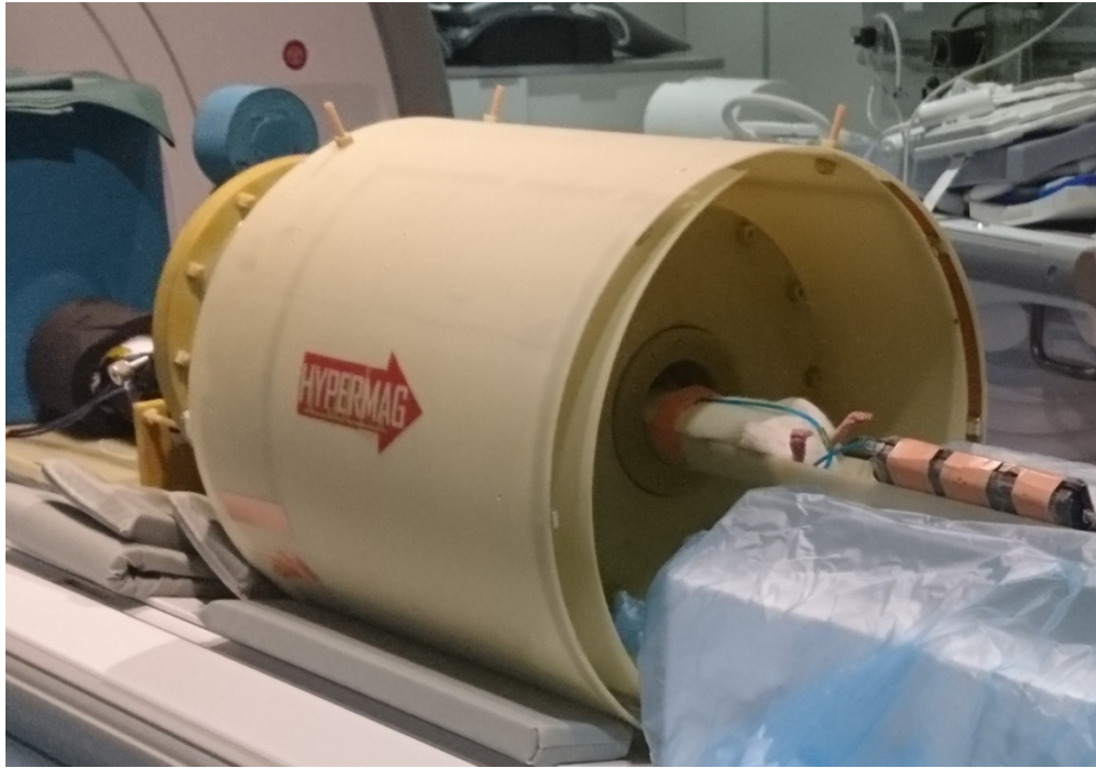
Figure 3. In-vivo experiments setup: the animal is placed in belly-up position to minimize the coil-to-brain distance, since the cryogenic coil is placed at the bottom part of the cryostat bore.
