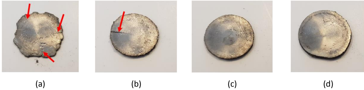
Fig. 23 Samples after uniaxial compression testing. The initial relative densities of the samples were (a) 72.0 %, (b) 86.6 %, (c) 90.3 % and (d) 96.0 %. Red arrows indicate the presence of cracks
