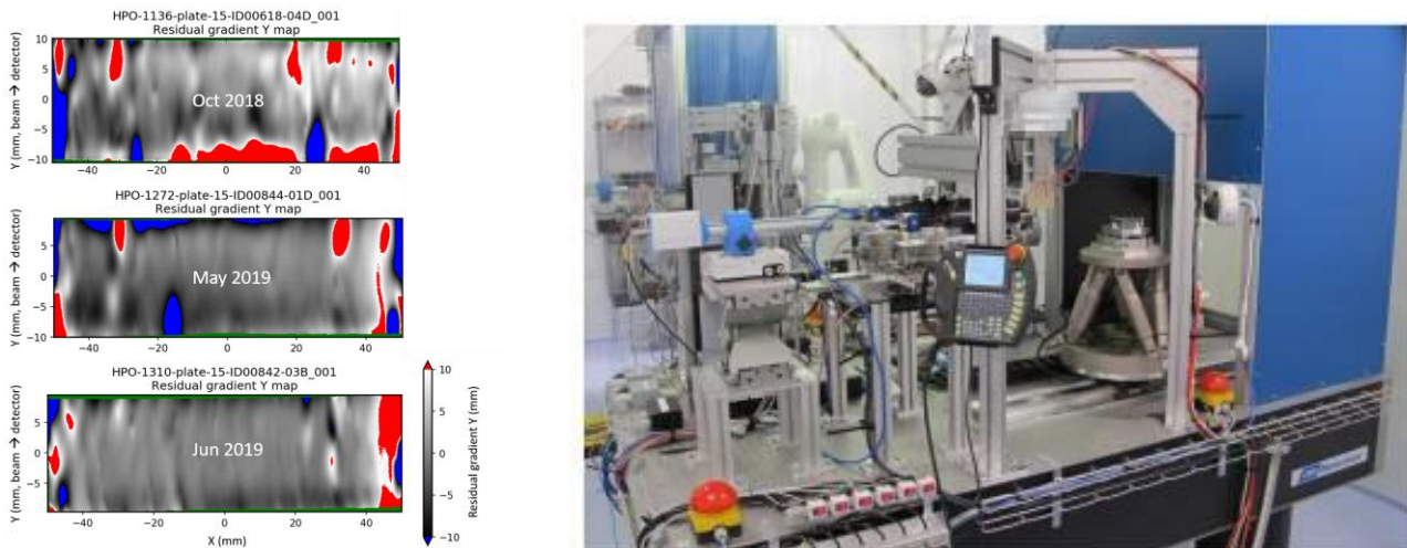
Figure 7: The left picture shows the evolution of the outer radius stack quality, comparing the FRT data of the 15 th plate of three stacks, as a function of time. The stacking recipe, developed on the middle radius robot, has been successfully migrated to the outer radius and significantly improved the quality of these stacks. The right picture shows a fourth stacking robot, developed and commissioned in 2019, which was installed in the cosine cleanroom. This robot will be dedicated for experimental work, whereas the other three robots are intended for continuous production on all three development radii.
