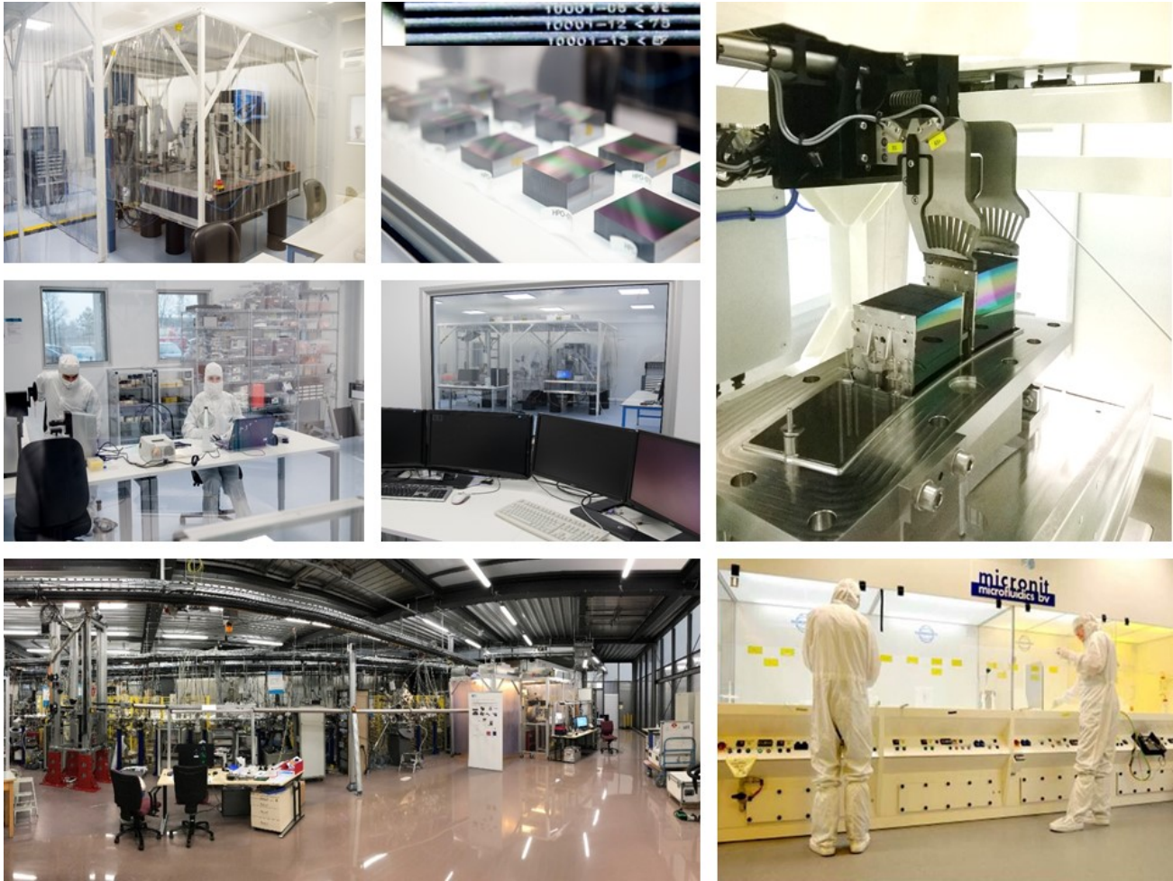
Figure 8: The production of the ATHENA optics is already largely automated and up-scalable for the production of the flight units. Clockwise from top left: stacking robot in clean tent inside the clean room, mirror plate stacks (insert showing individually labelled mirror plates), mirror modules being integrated into the optical bench, industrial facility used to produce mirror plates, X-ray beamline at the BESSY-II synchrotron facility, goods-incoming inspection cleanroom at cosine, and at the center: control room for stacking operations.
