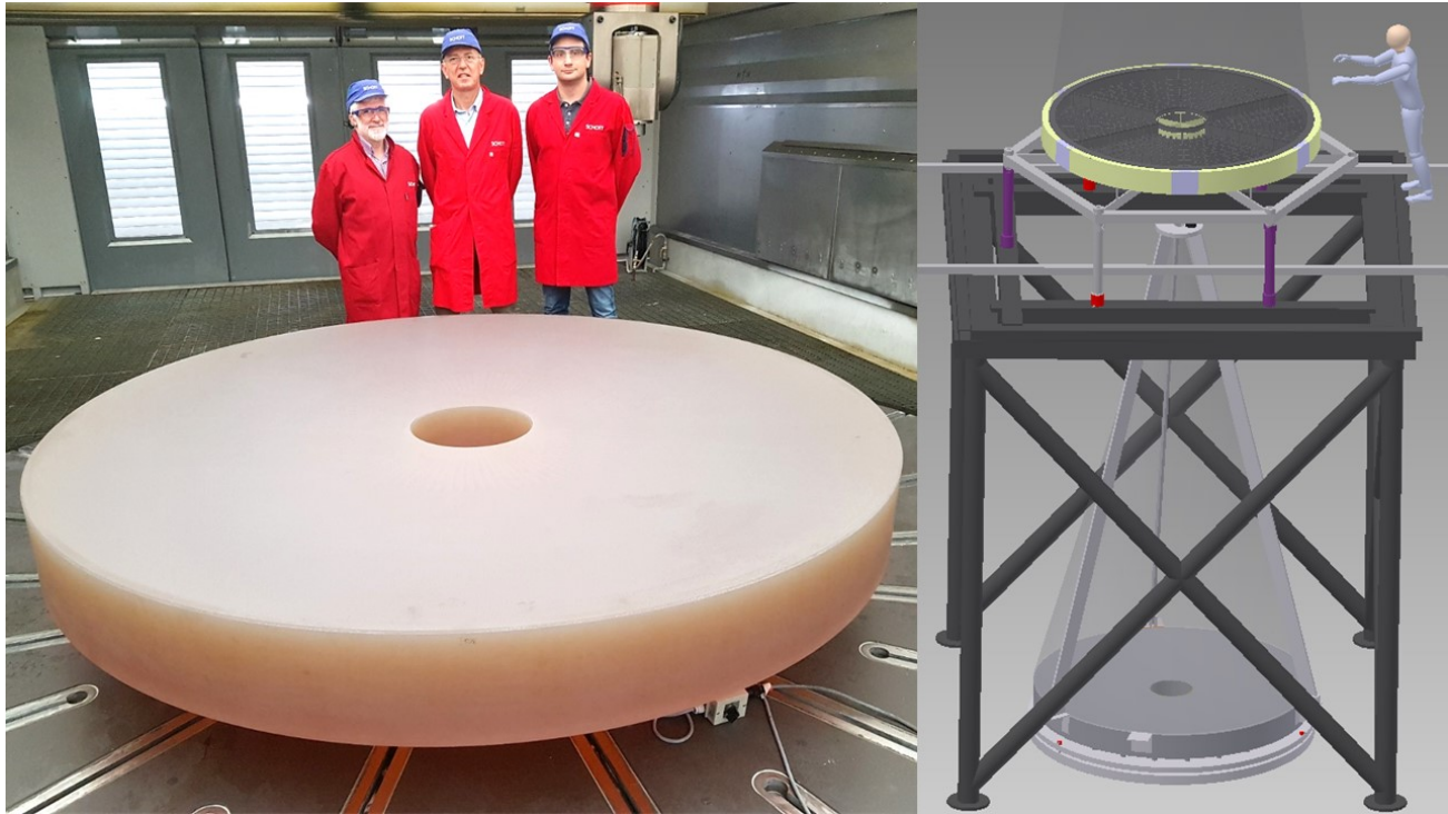
Figure 9: Left: Zerodur blank of 2.6 m diameter, machined by Schott AG to 50\ \mu\text{m} figure error, ready for shipment to Opteon Oy for lapping, polishing and final figuring. This long-lead item is a key element of the mirror module integration facility currently being implemented at Media Lario S.r.l. Right: sketch of the UV collimator using the 2.6 m mirror to produce a collimated vertical beam, serving to accurately position the mirror modules during integration into the Mirror Assembly Structure of ATHENA.
