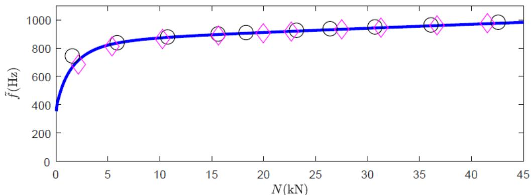
Figure 1: First transverse frequency of a bolt M12x260 as function of bolt tension. Solid line/markers: Theoretical/experimental results (adapted from [1]).
