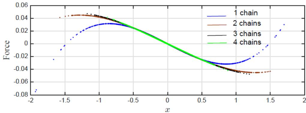
Figure 3: Correction part of the restoring force in the single-degree freedom spring-mass system.
