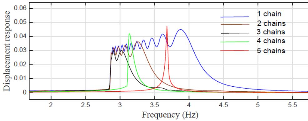
Figure 2: Fourier transform of the displacement impact response of the system for different numbers of chains.
