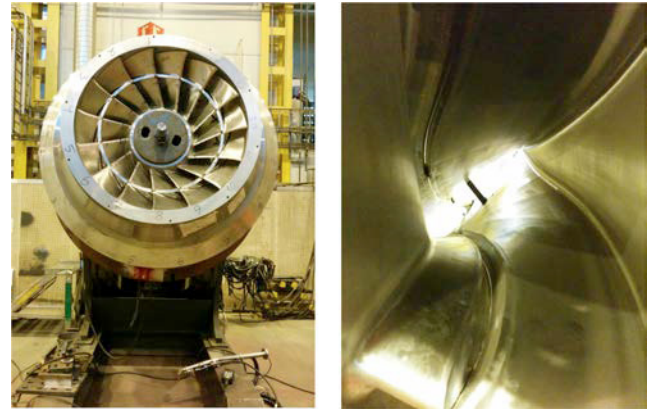
Fig. 1. A hydro-power water turbine with the welding grooves
