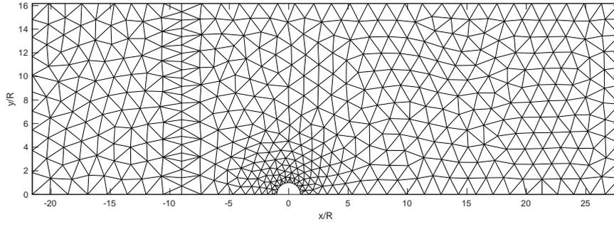
Figure 1: Illustration of mesh for the representation of the free surface plane. The mesh conforms with the interface of the wave generation zone (left part).
