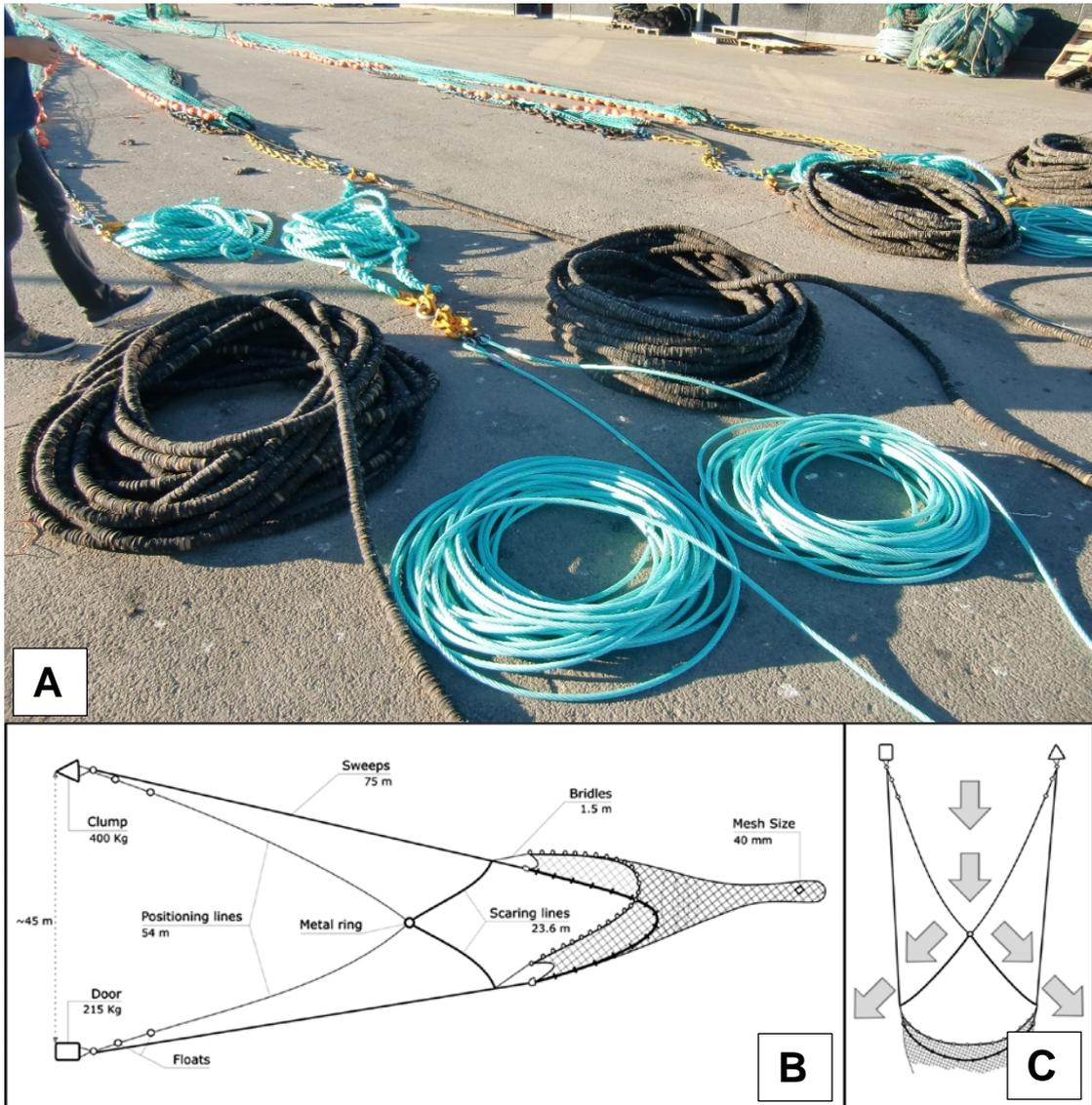
**Figure 4.** FLEXSELECT design. (A & B) The port trawl in a twin rig with FLEXSELECT mounted. Proportions are not respected to facilitate the identification of all FLEXSELECT components. (B) Desired counter-herding effect. The grey arrows represent the direction of fish escape.
