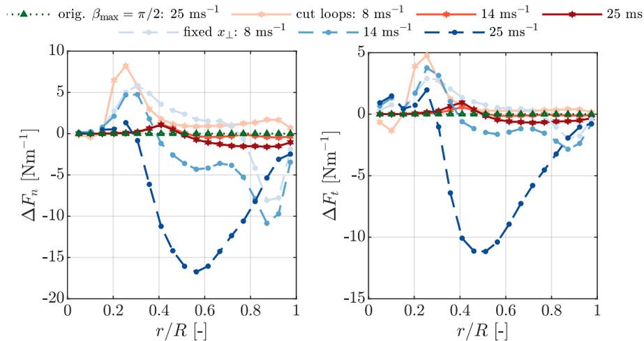
**Figure 2.** Difference in normal and tangential forces over the NREL 5MW blades at 8, 14 and 25  $\text{ms}^{-1}$  predicted by AL simulations (blades discretized by 19 sections) with different smearing correction speed-up methods with respect to simulations without speed-up.
