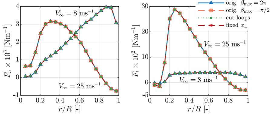
**Figure 1.** Normal and tangential forces on the NREL 5MW blades at 8 and 25  $\text{ms}^{-1}$  predicted by AL simulations (blades discretized by 19 sections) with smearing correction and different computational speed-up methods. The reference is the original formulation (orig.) with  $\beta_{\text{max}} = 2\pi$ .
