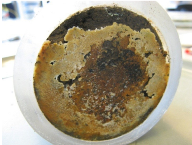
Figure 2: Cathode end of the soil sample after EDR of Soil 2.
