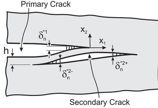
**Figure 1:** Delamination of a weak layer (secondary crack) at a distance  $h$  from the primary crack.  $\delta_n^{*1}$  is the normal end-opening of the primary crack,  $\delta_n^{*2-}$  and  $\delta_n^{*2+}$  the normal end-openings of the right and left hand side crack tips of the secondary crack. The corresponding tangential end-openings of the primary and secondary cracks are  $\delta_t^{*1}$ ,  $\delta_t^{*2-}$  and  $\delta_t^{*2+}$ .
