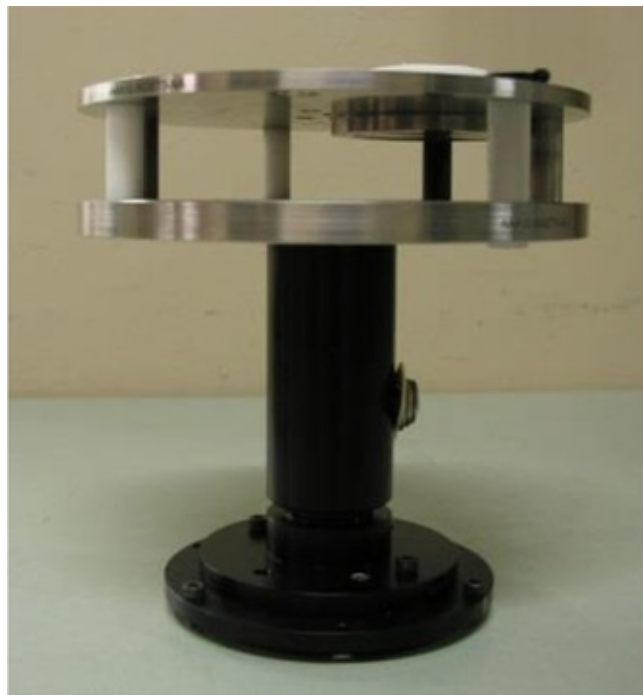
Figure 6.3: Picture of the carousel sample holder with six different materials in place. Figure courtesy of Dooraghi et al. [97]
