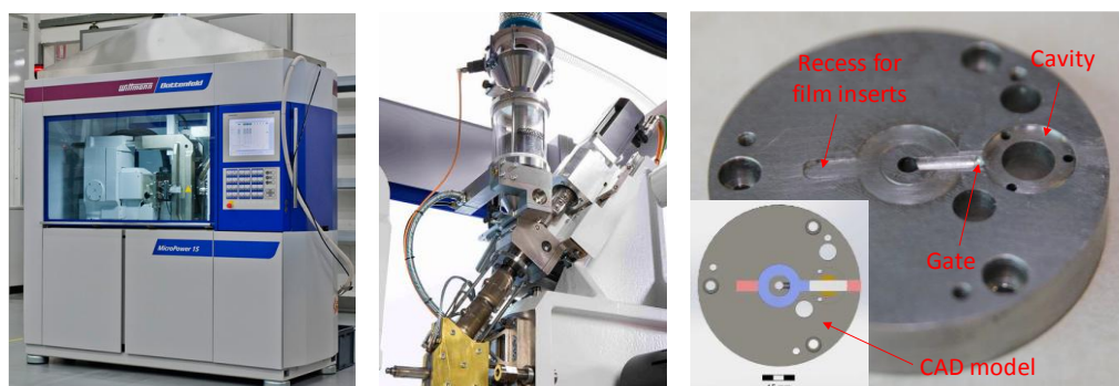
Figure 3. Wittmann–Battenfeld Micro Power 15 micro injection moulding machine used for the experiment (left), the injection unit of the of moulding machine (middle); and mould insert used in the tool to injection moulding of the FIM part (right).
