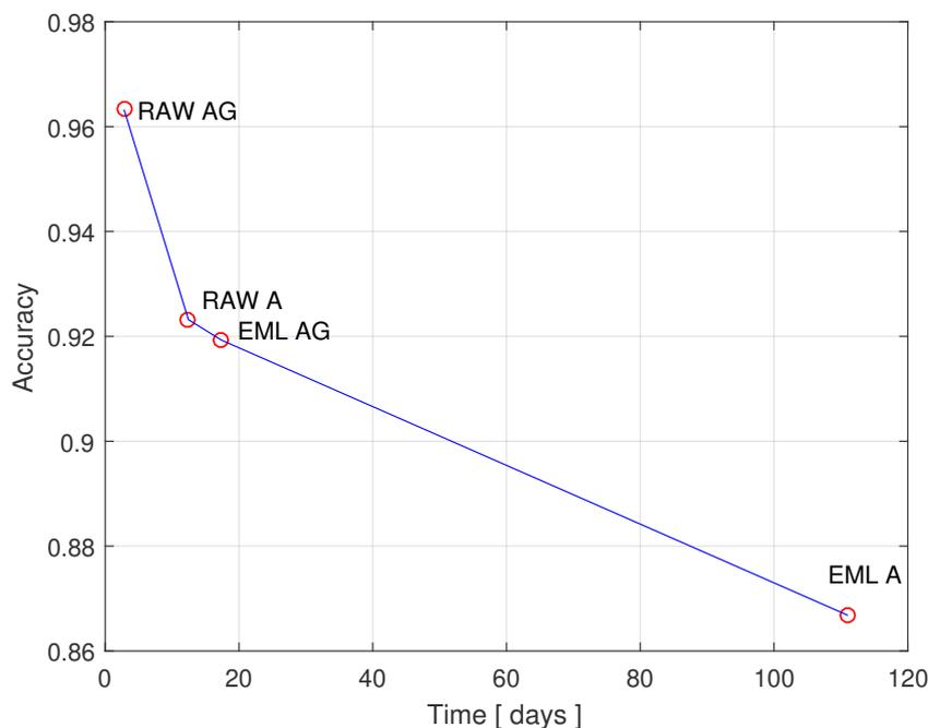
**Figure 5.** The trade-off between the model accuracy and lifetime. Legend: Raw Data—Accelerometer Only (RAW A); Raw Data—Accelerometer and Gyroscope (RAW AG); On-Board Classification—Accelerometer Only (EML A); On-Board Classification—Accelerometer and Gyroscope (EML AG).
