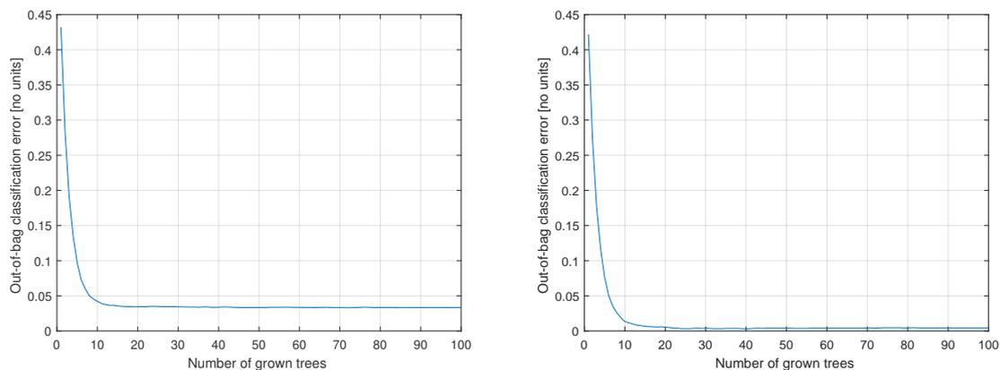
**Figure 3.** The effect of decreasing the number of trees on the accuracy of the Stage 1 classifier (**left**) and Sedentary classifier (**right**). 10 trees is a reasonable compromise between accuracy and feasibility for on-board implementation.
