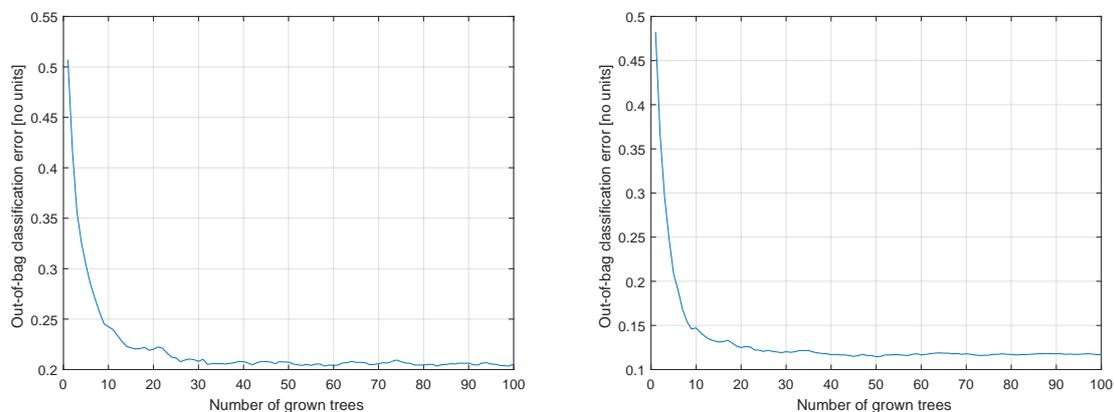
**Figure 4.** The effect of decreasing the number of trees on the accuracy of the Moderate classifier (**left**) and Rigorous classifier (**right**). 10 trees is a reasonable compromise between accuracy and feasibility for on-board implementation.
