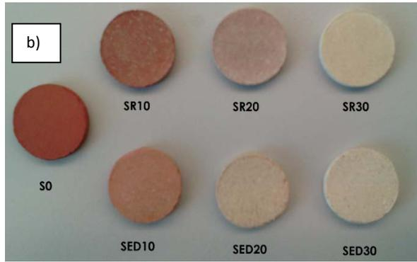
Fig. 3 Colours of discs with substitution of clay with different amounts (0%, 10%, 20%, 30%) fly ash (R – raw, ED – treated). a) Teglværk (T) clay discs, b) Sisimiut (S) clay discs.
