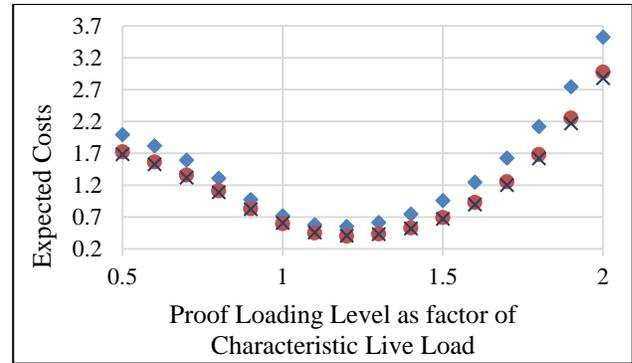
Figure 4: Illustration of the Expected Costs given  $Z_1$  from the two monitoring strategies  $i_1$  (orange circle) and  $i_2$  (blue cross) and the expected costs with only loading ' $U(S_{PL_j})$ ' (blue diamond) as a function of the loading level.
