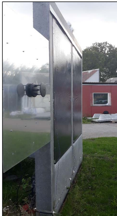
Fig. 3: Location of the ultrasonic wind sensor.
