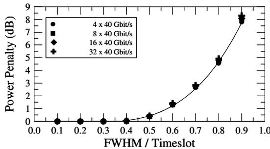
**Figure 2.18:** Power penalty for multiplexing and demultiplexing ideal Gaussian transform-limited pulses with no pedestal.
