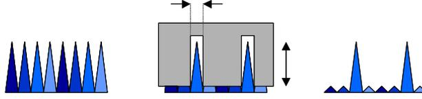
**Figure 4.13:** Variation of width, extinction ratio and shape of SW and the impact on the demultiplexed signal.
