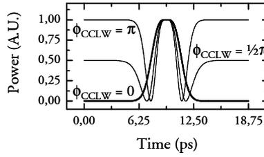
**Figure 4.28:** CW light with power of 1 switched in NOLM controlled by Gaussian control pulse for  $\phi_{\text{CCLW}}$  varied from 0 to  $\pi$  in steps of  $\frac{1}{2}\pi$ . Phase difference at peak of SW  $\Delta\phi = (\phi_{\text{CLW}} - \phi_{\text{CCLW}}) = \pi$ .
