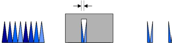
**Figure 4.15:** Illustration of the effect of timing jitter on the clock controlling the temporal position of the SW.
