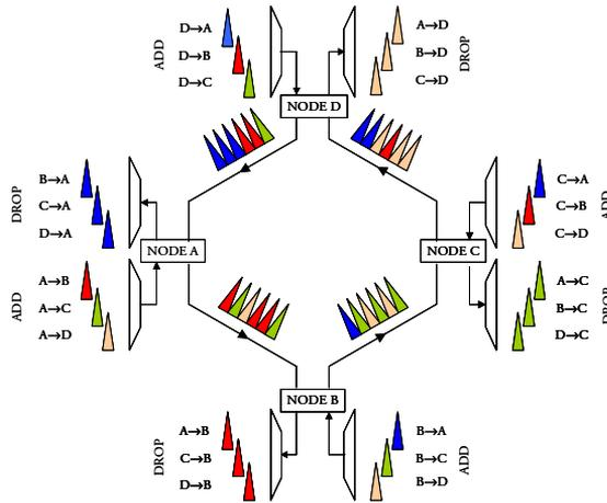
**Figure 5.24:** OTDM network with full connectivity based on an uni-directional ring with 4 nodes.
