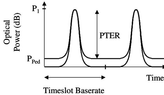
**Figure 2.13:** Definition of Pulse Tail Extinction Ratio for pulses with an additional pedestal.
