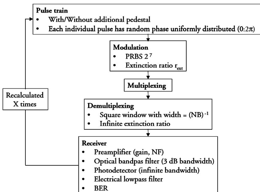
Figure 2.16: Diagram of power penalty simulations for different pulses.
