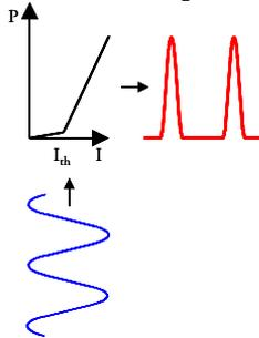
Figure 2.3: Simple illustration of the principle behind gain-switching of a laser.
