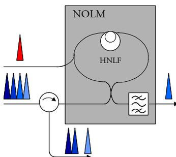
Figure 4.9: Principle of switching using a NOLM
