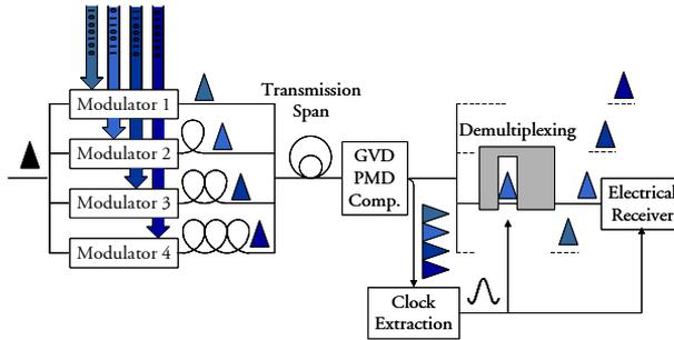
Figure 3.1: Basic bit-interleaved OTDM point-to-point transmission system
