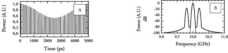
**Figure 5.13:** (A) 10 GHz pulse train pilot tone modulated with modulation index  $m = 0.3$ . (B) Spectrum of pulse train without pilot tone modulation (thin line) and with pilot tone modulation (bold line).
