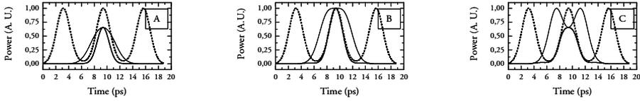
**Figure 4.32:** Impact of phase-difference  $\Delta\phi$  on a 160 GHz switched pulse train.  $\Delta\phi = 0.6\pi$  (A).  $1.0\pi$  (B) and  $1.4\pi$  (C) with  $\alpha = 0.50$  and  $\phi_{\text{CCLW}} = 0$ . Dashed line is 160 GHz pulse train with FWHM =  $0.4T_s$ . Thin line is SW of NOLM, with FWHM of the Gaussian phase variation of  $0.6T_s$  corresponding to optimum performance for  $\Delta\phi = 1.0\pi$ . Bold line is demultiplexed signal.
