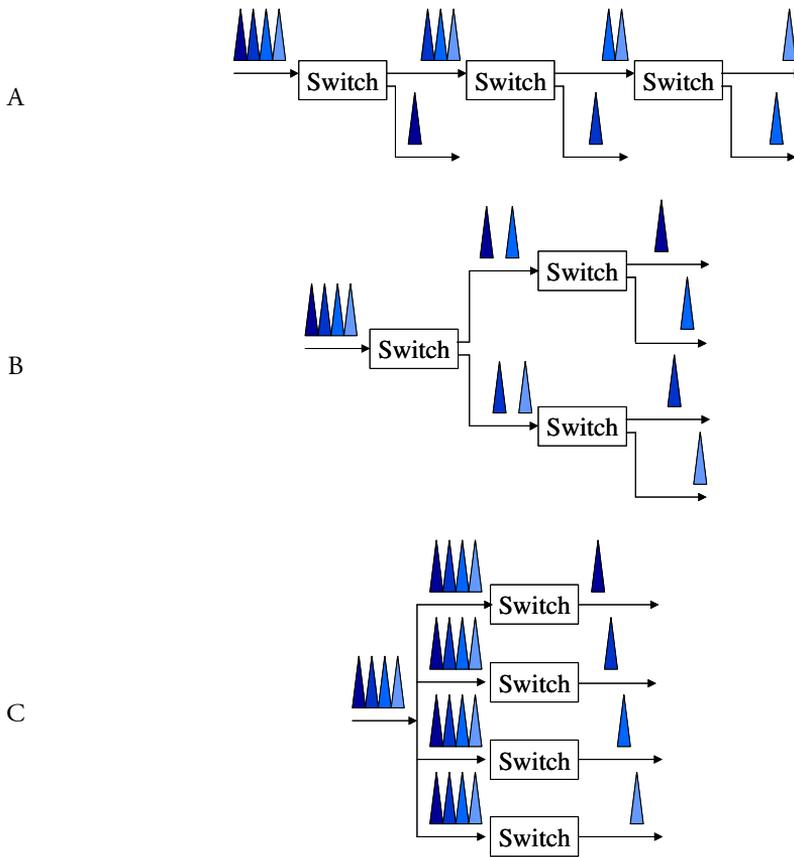
**Figure 4.3:** Different demultiplexing structure implementations for a point-to-point OTDM system. A) Serial structure B) Tree structure C) Parallel structure.
