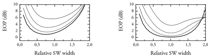
**Figure 4.25:** EOP as function of FWHM SW width evaluating the impact of SW offset. Offset is increased from  $0.0T_s$  (bold line) to  $0.4T_s$ . OTDM signal based on pulses with FWHM =  $0.4T_s$  is demultiplexed with Gaussian (left) and Super Gaussian (right) switch.
