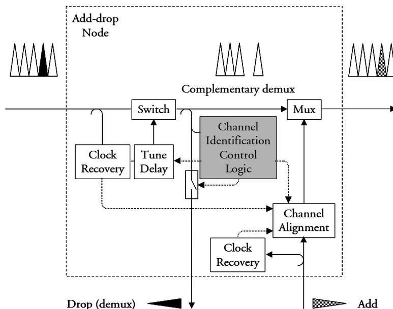
Figure 5.5: Optical Add Drop Multiplexer (OADM) node, showing some of the required functionalities required in order to drop target channel and add a new time channel in the empty time slot.
