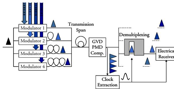
**Figure 1.1:** Point-to-point bit interleaved Optical Time Division Multiplexed (OTDM) system
