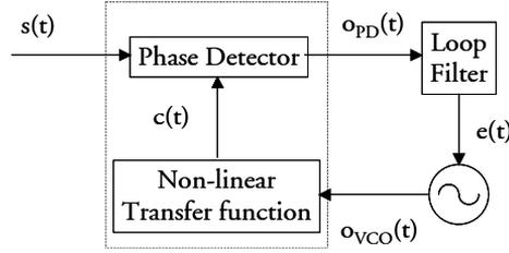
**Figure 3.4:** PLL configuration for accommodating base rate clock extraction from an OTDM signal
