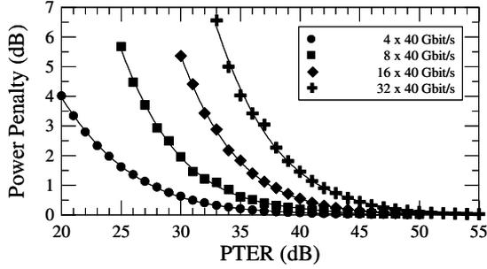
**Figure 2.20:** Power penalty versus PTER for pulse width FWHM equal to 0.3 times the width of the OTDM timeslot. The 1 dB penalty is obtained for PTER equal to 27, 33, 37 and 41 dB, for 160, 320, 640 and 1280 Gbit/s respectively.
