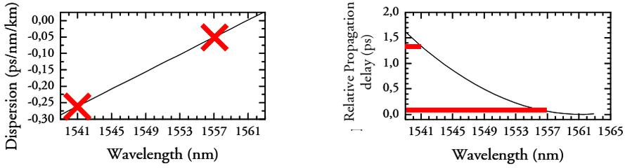
**Figure 4.36:** Dispersion as function of wavelength for 500 m of HNLF used for 320 to 10 Gbit/s demultiplexing (left). Relative propagation delay as function of wavelength (right). Crosses and lines correspond to values for control and data signals.
