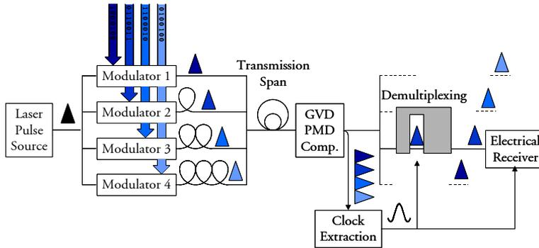
Figure 4.1: Basic OTDM point-to-point communication system.
