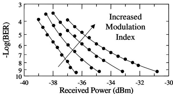
Figure 5.21: Experimentally measured BER curves for data signal applied pilot tone modulation with a modulation index  $m$  of 0.00, 0.39, 0.53 and 0.59.
