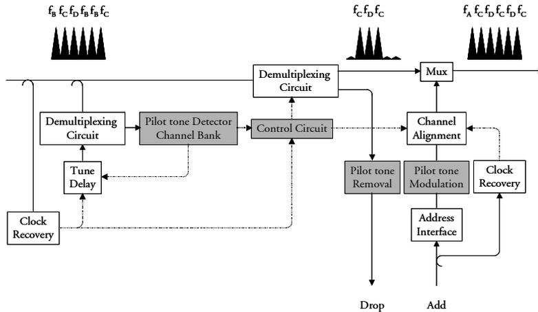
**Figure 5.29:** Proposed structure of an OADM allowing for dynamical allocation of the channels, based on the pilot tone scheme.
