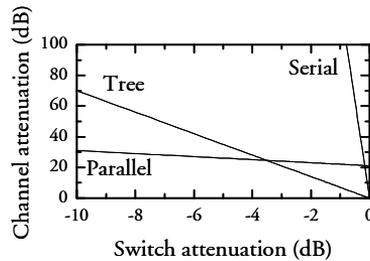
**Figure 4.4:** Channel attenuation as function of switch attenuation for OTDM signal based on 128 aggregated channels (worst-case).
