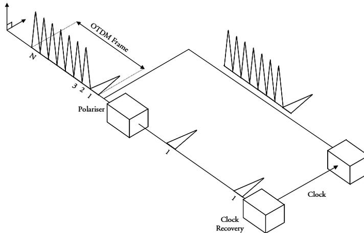
**Figure 5.8:** OTDM signal composed by  $N$  channels. The SOP of channel 1 is perpendicular to the other  $(N-1)$  channels.
