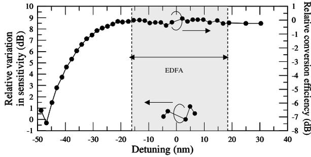
**Figure 2.10:** Relative variation in sensitivity, relative conversion efficiency for HNLF and EDFA gain bandwidth (-1535-1570 nm) (marked as grey box) all as function of detuning.
