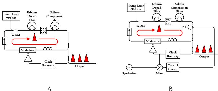
**Figure 2.5:** A) shows the principle of a regenerative ML-FRL. B) A regenerative ML-FRL offering the possibility for external synchronisation [2.20].
