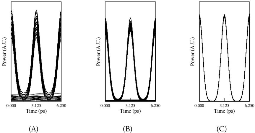
**Figure 2.19:** Eye-diagrams for 320 Gbit/s signal with pulses with FWHM pulse widths of 0.9373 ps (0.3 times the timeslot) and with PTER of A) 25 dB, B) 33 dB and C) 50 dB.
