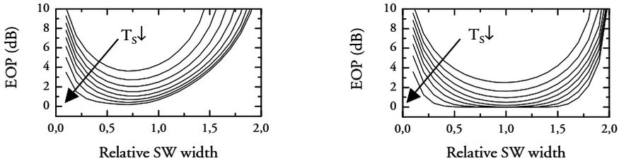
**Figure 4.20:** EOP2 depicted as function of relative SW width using Gaussian (left) and Super Gaussian (right) SW for demultiplexing OTDM signals based on pulse trains with relative FWHM equal to 0.1 to 0.9 times the OTDM time slot  $T_s$ .
