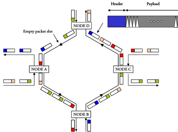
Figure 5.30: Uni-directional ring based on packet switching.
