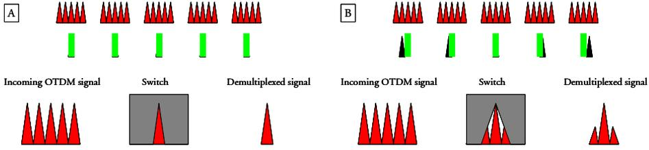
**Figure 4.34:** Graphic illustration of no walk-off (A) and with walk-off (B) on the switching performance. Square box indicates matched alignment position between control and OTDM data signal.
