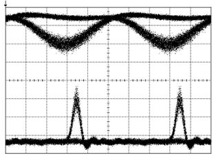
Figure 4.39: 10 Gbit/s demultiplexed electrical (upper trace) and the optical (lower trace) eye-diagrams corresponding to the sensitivity at the BER =  $10^{-9}$ .
