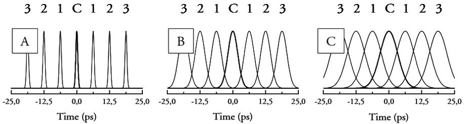
**Figure 2.17:** Electric field of a 160 GHz pulse train based on Gaussian pulses. The numbers refer to the number from the central channel C. A)  $T_{\text{FWHM}}$  equal to 0.1 of the timeslot  $T_s$ , i.e. 0.625 ps. B)  $T_{\text{FWHM}}$  equal to 0.5 of the timeslot  $T_s$ , i.e. 3.125 ps. C)  $T_{\text{FWHM}}$  equal to 0.9 of the timeslot  $T_s$ , i.e. 5.625 ps.
