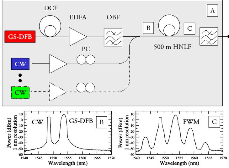
**Figure 2.9:** A) Principle set-up for wavelength converting a pulse train. B) Optical spectrum at the input to the HNLF. C) Optical spectrum at the output of the HNLF containing the generated FWM product.
