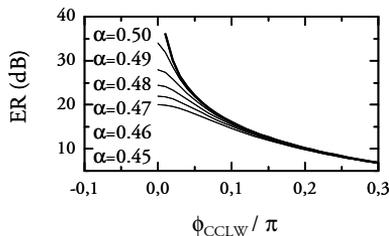
**Figure 4.30:** ER plotted as function of the ratio  $\phi_{\text{CCLW}}/\pi$  for  $\alpha$  varied from 0.50 to 0.45 in steps of 0.01
