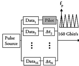
**Figure 5.10:** OTDM Transmitter including one branch with additional modulator for applying amplitude modulation serving as the pilot tone. The frequency of the pilot tone is  $f_p$
