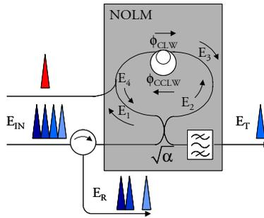
**Figure 4.26:** NOLM introducing the parameters used to describe the simplified model below
