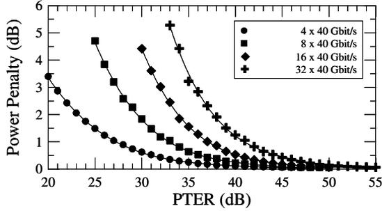
**Figure 2.21:** Power penalty versus PTER for pulse width FWHM equal to 0.4 times the width of the OTDM timeslot. The 1 dB penalty is obtained for PTER equal to 27, 33, 37 and 41 dB, for 160, 320, 640 and 1280 Gbit/s respectively.
