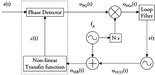
**Figure 3.14:** Suggested configuration 3 for compensating DC component. Notice the symbol  $\oplus$  in this configuration represents Single Sideband Modulation of the oscillator frequency.
