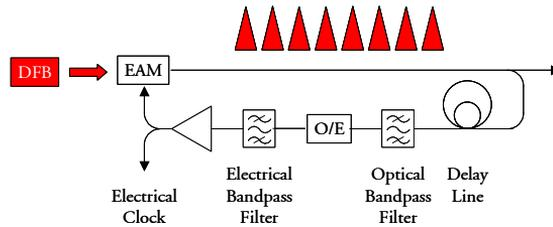
Figure 2.8: Pulse source based on injection locking of EAM [2.33].
