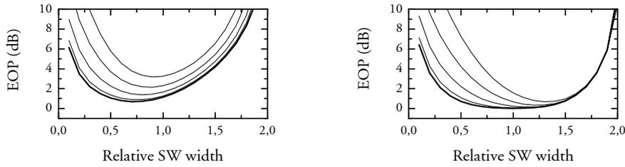
**Figure 4.22:** EOP as function of FWHM SW width, evaluating the impact of offset of the target channel. Offset is increased from  $0.0T_s$  (bold line) to  $0.4T_s$ . OTDM signal based on pulses with  $\text{FWHM} = 0.4T_s$  is demultiplexed with Gaussian (left) and Super Gaussian (right) switch.
