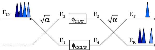
**Figure 4.27:** Conceptual description of NOLM operation by symbolising the Sagnac interferometer with a Mach-Zehnder representation.
