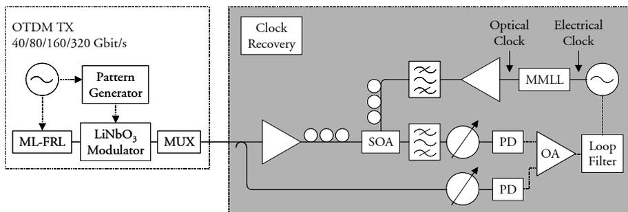
**Figure 3.20:** Experimental set-up for extracting a 10 GHz clock from 40, 80, 160 Gbit/s. ML-FRL: Mode-locked Fibre Ring Laser. Mux: Multiplexer. SOA: Semiconductor Optical Amplifier. PD: Photo-Detector. OA: Operational Amplifier. MMLL: Monolithic mode-locked Laser.
