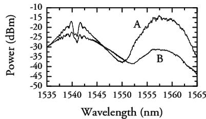
**Figure 4.37:** Spectra of control and data signal measured at point A and B (see Figure 4.35).
