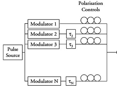
Figure 5.7: OTDM transmitter including polarisation controls in each branch.
