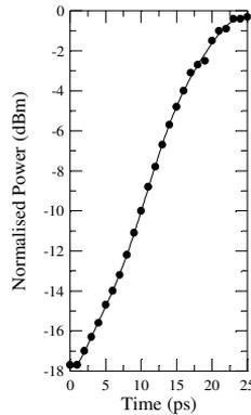
**Figure 5.23:** Normalised pilot tone power as function relative position of SW to data signal.
