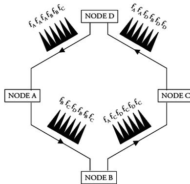
**Figure 5.28:** OTDM ring network based on uni-directional ring, with pilot tone identification.
