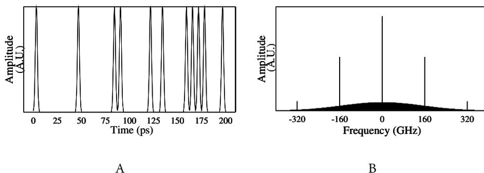
Figure 3.7: (A) pattern of 160 Gbit/s signal with PRBS  $2^7-1$  (B) corresponding spectrum
