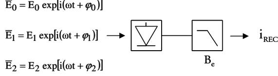
**Figure 2.12:** Example for illustrating crosstalk in OTDM systems. Three electric fields are injected into a photo-detector, before filtering in a lowpas filter.
