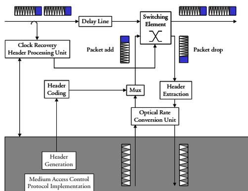
**Figure 5.31:** Access node in Optical Packet Compression Time Division Multiplexed system, based on [5.21].
