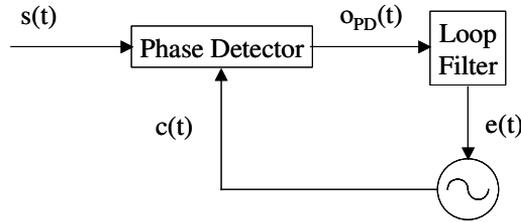
**Figure 3.3:** Basic Phase Locked Loop (PLL) configuration
