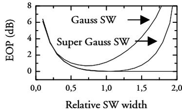
**Figure 4.19:** EOP1 and EOP2 as function of relative FWHM SW width for an OTDM system based on pulses with FWHM equal to  $0.4T_s$  and demultiplexed using a switch with Gaussian and Super Gaussian shaped SW. EOP1 is identical for the two switches.
