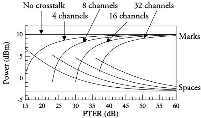
**Figure 2.14:** Example of worst-case crosstalk scenario for an input signal with +10 dBm in mark and modulation extinction ratio of 13 dB. The crosstalk is calculated for 4, 8, 16 and 32 channel OTDM signal.
