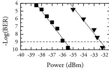
Figure 4.38: BER measurements for 10 Gbit/s back-to-back configuration based on compressed pulses and after 320 to 10 Gbit/s demultiplexing.
