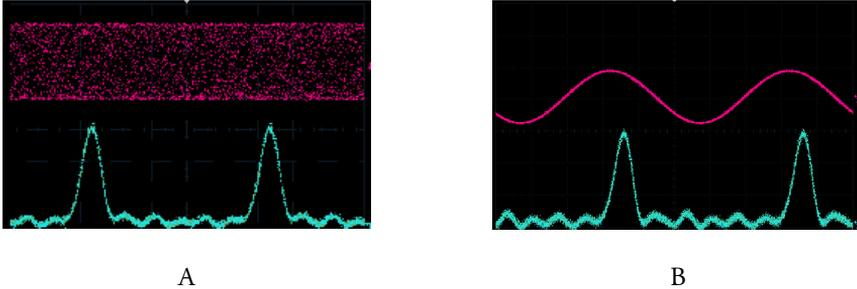
**Figure 3.22:** A) Upper trace shows unlocked clock. Lower trace the base rate optical pulse train. B) Upper trace shows locked clock extracted from 80 Gbit/s. Lower trace identical to lower trace A).
