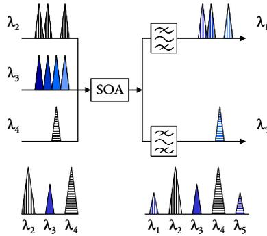
**Figure 4.8:** Generation of demultiplexed and complementary demultiplexed signal using FWM in SOA [4.47]
