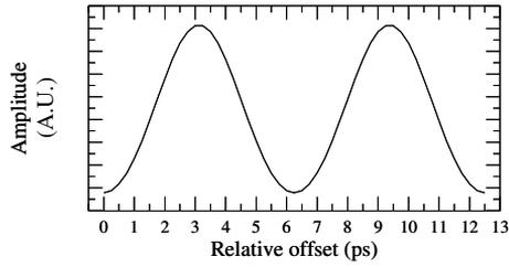
**Figure 3.9:** Control signal for PLL as function of relative offset between OTDM signal and clock pulse train
