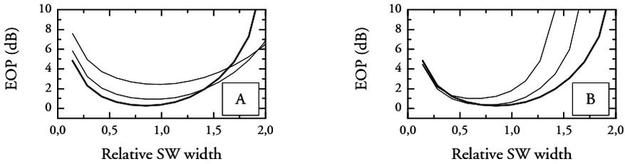
**Figure 4.31:** Impact of phase-difference  $\Delta\phi$  variation. Power splitting ratio  $\alpha = 0.50$ , the counter clockwise phase-shift  $\phi_{\text{CCLW}} = 0$ . In A,  $\phi_{\text{CLW}}$  is varied from  $0.6\pi$ ,  $0.8\pi$  and  $1.0\pi$  and in B,  $\phi_{\text{CLW}}$  is varied from  $1.0\pi$ ,  $1.2\pi$  and  $1.4\pi$ .
