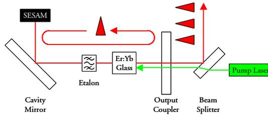
Figure 2.6: Illustration of the principle behind the ERGO laser [2.28].
