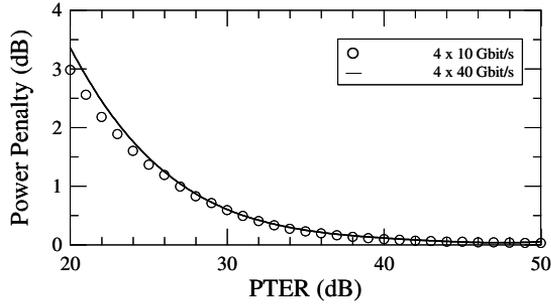
**Figure 2.15:** Comparison of induced power penalty versus PTER for a 4 x 10 Gbit/s system (o) and a 4 x 40 Gbit/s (-).
