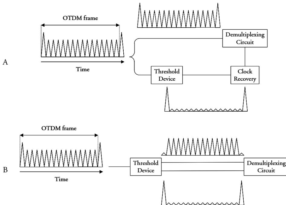
**Figure 5.9:** Modified OTDM signal, by increasing the peak power of channel 1 compared to the other  $(N-1)$  channels. A) Corresponds to the suggested set-up in [5.7] and B) to the set-up in [5.8].
