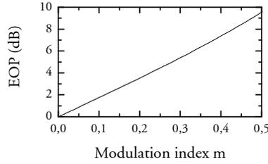
Figure 5.16: EOP as function of modulation index m of pilot tone modulation
