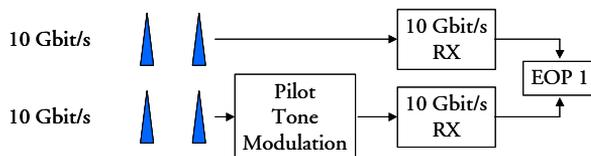
**Figure 5.15:** Principle of EOP simulations addressing impact of modulation index  $m$  of the pilot tone modulation
