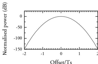
**Figure 5.14:** Power of discrete pilot tone as function of detuning between the centre of the pilot tone modulated channel and the Switching Window.
