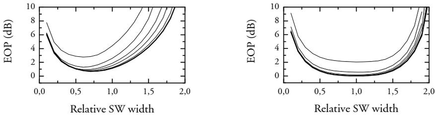
**Figure 4.21:** EOP as function of FWHM width of SW. ER varied from infinite (bold lines) to 30, 20, 15, 10 and 5 dB. SW is Gaussian (left) and Super Gaussian (right).
