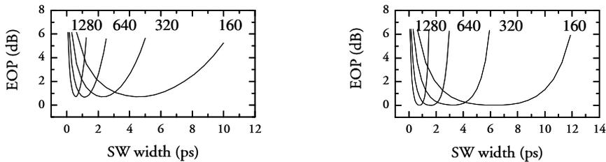
**Figure 4.18:** Demultiplexing of 160, 320, 640 and 1280 Gbit/s OTDM signals in a switch, with Gaussian (left) and Super Gaussian (right) shaped SW is evaluated by calculating the EOP. Pulses of the data pulses correspond to 0.40 times the OTDM time slot. The width of the SW is varied.
