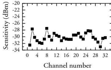
**Figure 4.40:** Sensitivity measured for all time channels constituting the 320 Gbit/s signal.
