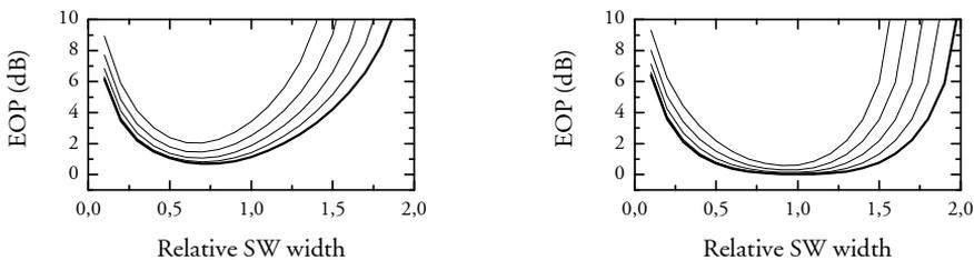
**Figure 4.24:** EOP as function of FWHM SW width, evaluating the impact of offset moving the neighbouring channels towards target channel and the target channel moved with the same offset away from the ideal timing position. Offset is increased from  $0.0T_s$  (bold line) to  $0.2T_s$  in steps of  $0.05T_s$ . OTDM signal based on pulses with FWHM =  $0.4T_s$  is demultiplexed with Gaussian (left) and Super Gaussian (right) switch.
