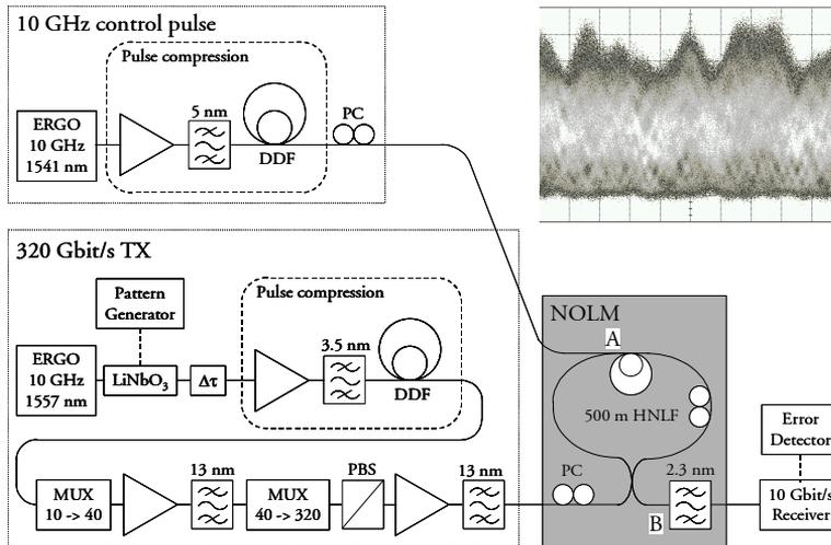
**Figure 4.35:** Experimental set-up for generating and demultiplexing the 320 Gbit/s OTDM signal. The inset shows the eye-diagram of the 320 Gbit/s signal.
