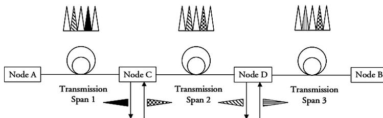
**Figure 5.4:** OTDM network including additional intermediate nodes based on Optical Add-Drop Multiplexing.
