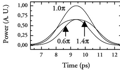
**Figure 4.33:** Comparison of 160 GHz switched signals for  $\Delta\phi = 0.6\pi$ ,  $1.0\pi$  and  $1.4\pi$  with  $\alpha = 0.50$ ,  $\phi_{\text{CCLW}} = 0$  and FWHM of Gaussian phase-change =  $0.6T_s$ .
