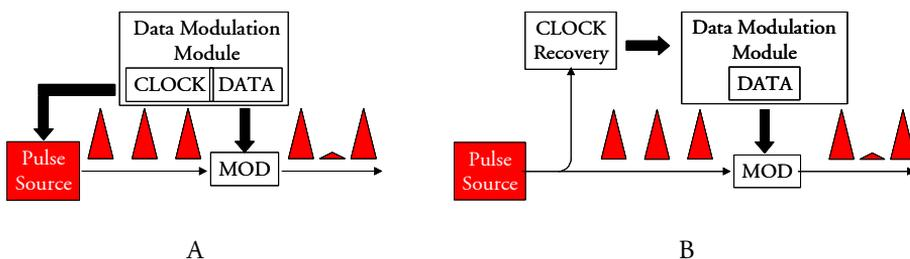
Figure 2.2: Two approaches for synchronising pulse source and data modulation module.
