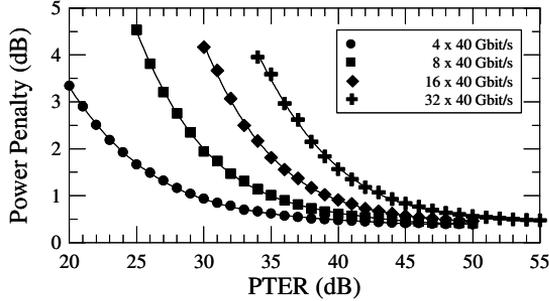
**Figure 2.22:** Power penalty versus PTER for pulse width FWHM equal to 0.5 times the width of the OTDM timeslot. The 1 dB penalty is obtained for PTER equal to 29, 35, 37 and 43 dB, for 160, 320, 640 and 1280 Gbit/s respectively.
