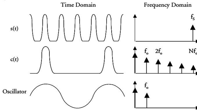
**Figure 3.5:** The impact of the non-linear transfer function used to introduce frequency components in the clock signal at the data frequency  $f_s$ , which corresponds to the aggregated bit rate of the OTDM signal composed by  $N$  time channels with base rate frequency of  $f_B$ .
