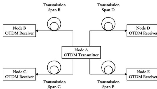
**Figure 5.3:** Star architecture based on OTDM technology used for broadcasting
