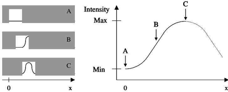
**Figure 3.2:** Principle of operation for an OPD. The output power of the OPD is a function of the relative position between the Switching Window (in grey) and the data signal.
