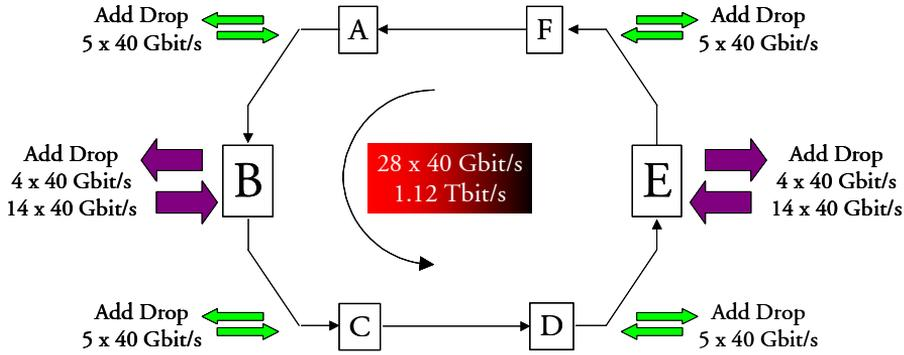
Figure 5.27: OTDM uni-directional ring network of heterogeneous users
