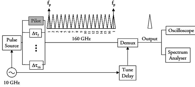
Figure 5.12: Numerical set-up used to evaluate the pilot tone scheme.
