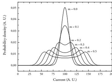
**Figure 5.17:** Probability density for a received mark, with pilot tone modulation  $m$  varied from 0.0 to 0.5 in steps of 0.1.
