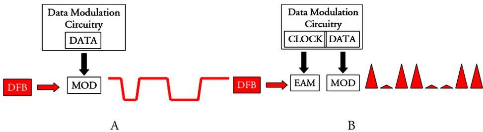
Figure 2.7: The upgrade from NRZ (A) to RZ (B) format using an EAM
