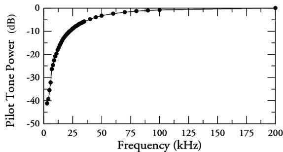
**Figure 5.18:** Pilot tone power after an EDFA as function of the pilot tone frequency  $f_p$ . The 3 dB cut-off frequency is approximately 55 kHz.
