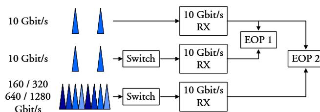
Figure 4.17: Calculation of EOP1 and EOP2 evaluating the impact of the switching window used for demultiplexing.
