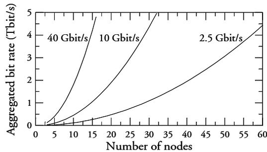
**Figure 5.25:** Aggregated bit rate in the OTDM network as function of the number of nodes for base rate varied from 2.5, 10 and 40 Gbit/s
