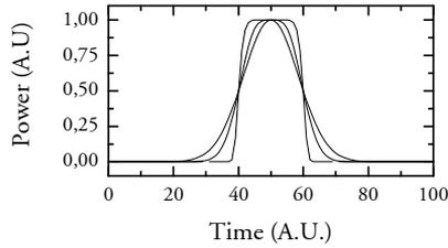
**Figure 4.14:** Example of three different switching windows evaluated. The steepest slope is the Super Gaussian SW (order  $m = 5$ ), followed by the simple NOLM model and finally the Gaussian SW.
