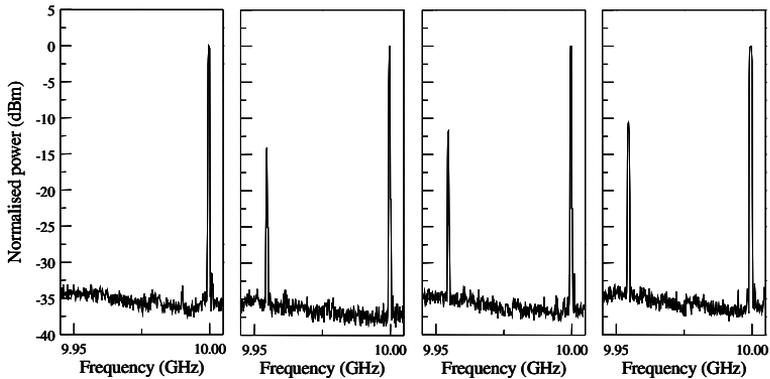
Figure 5.20: Zoom on the experimentally measured electrical spectra of data signals applied pilot tone modulation with modulation index  $m$  ranging from 0.00, 0.39, 0.53 and 0.59, starting from left to right.
