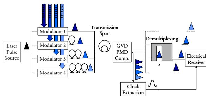
Figure 2.1: Basic OTDM communication system.
