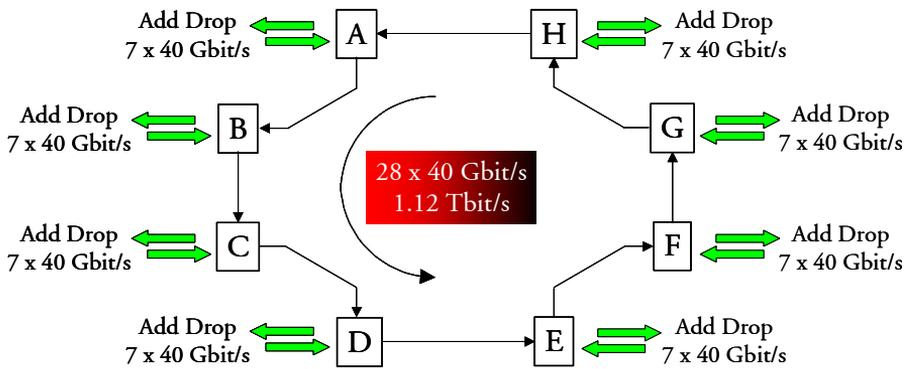
Figure 5.26: OTDM uni-directional ring network of homogenous users
