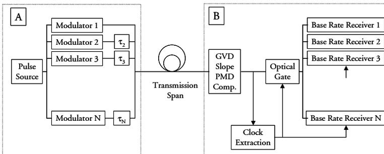
Figure 5.1: OTDM system used for point-to-point transmission.
