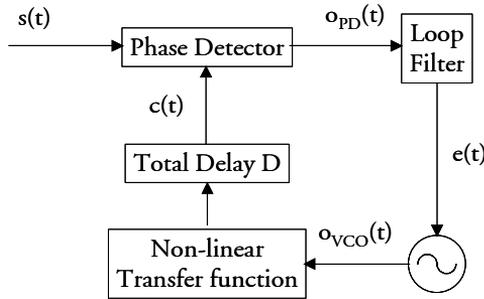
Figure 3.17: Modified PLL configuration including a total loop delay D
