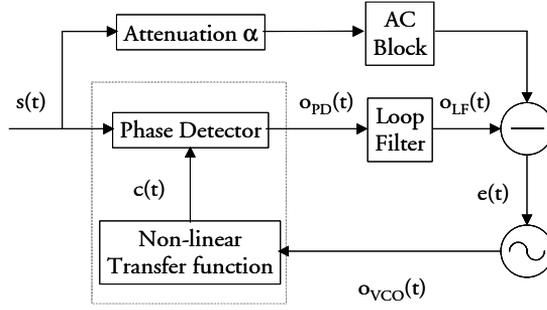
**Figure 3.13:** Suggested configuration 2 for compensating DC component
