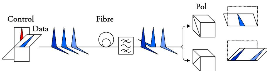
Figure 4.10: Principle behind Kerr switching
