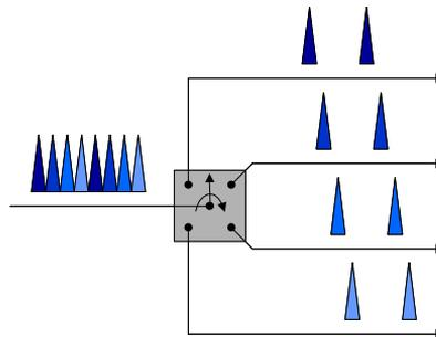
Figure 4.2: Principle of switch in OTDM system
