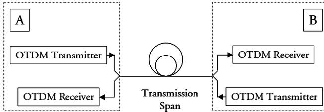
**Figure 5.2:** Two parallel OTDM systems used to allow for bi-directional transmission.
