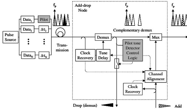
Figure 5.11: Pilot tone scheme implemented in an OTDM network.
