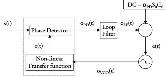
Figure 3.11: Suggested configuration 1 for compensating DC component
