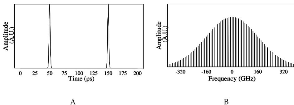
Figure 3.8: (A) pattern of 10 GHz Gaussian pulse train (B) corresponding spectrum
