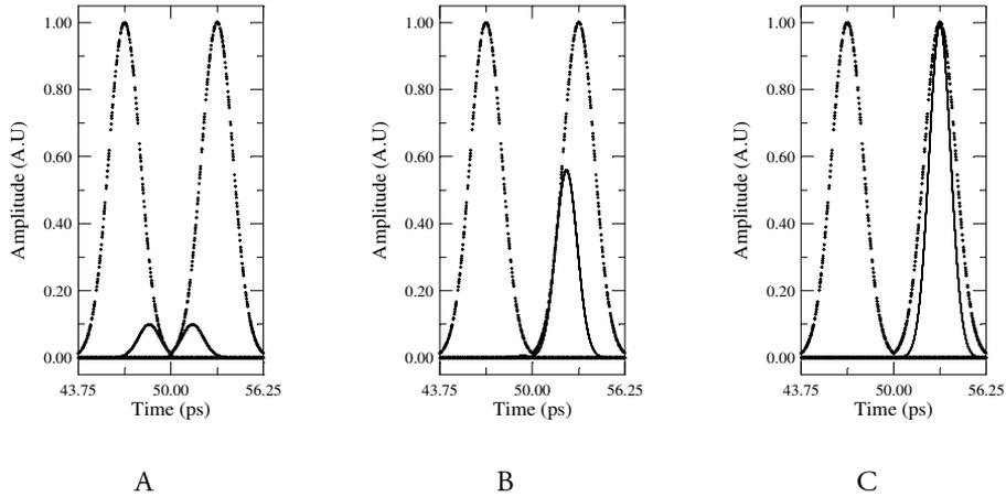
**Figure 3.10:** 160 Gbit/s data signal (dotted lines) multiplied a clock pulse. The output of the optical switch (full line) is calculated for 3 different situations A) Out-of-phase B) Phase quadrature and C) In-phase
