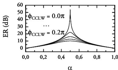
**Figure 4.29:** Extinction Ratio in dB as function of  $\alpha$  for  $\phi_{\text{CCLW}}$  values varied from 0 to  $0.2\pi$  in steps of  $0.05\pi$ . For increased  $\phi_{\text{CCLW}}$  the ER drops.
