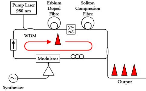
Figure 2.4: Actively Mode-Locked Fibre Ring Laser
