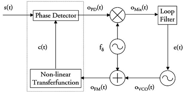
**Figure 3.15:** Suggested configuration 4 for compensating DC component. Notice the symbol  $\oplus$  in this configuration represents Frequency Modulation of the oscillator frequency.
