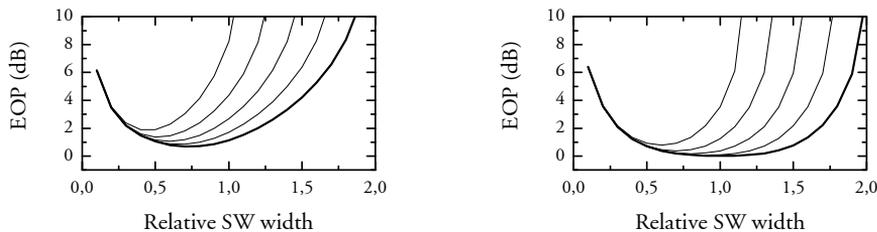
**Figure 4.23:** EOP as function of FWHM SW width, evaluating the impact of offset of neighbouring channels towards target channel. Offset is increased from  $0.0T_s$  (bold line) to  $0.4T_s$  in steps of  $0.1T_s$ . OTDM signal based on pulses with  $\text{FWHM} = 0.4T_s$  is demultiplexed with Gaussian (left) and Super Gaussian (right) switch.
