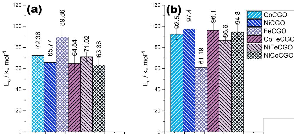
Figure 4. The averaged activation energy measured in  $\text{kJ} \cdot \text{mol}^{-1}$  in a) 4% H<sub>2</sub>O/H<sub>2</sub> and in b) 50% H<sub>2</sub>O/H<sub>2</sub>. Notably, the metal catalyst loading of the pure metal infiltrated cells, are 10 times higher than the cells, which have been co-infiltrated with CGO.
