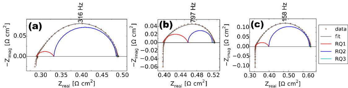
Figure 2. Fitting of the equivalent circuit L-R-RQ-RQ-RQ, for a) a Co-Fe-CGO symmetrical cell, b) a Ni-Co-CGO symmetrical cell, and c) a Ni-Fe-CGO symmetrical cell in 50% H<sub>2</sub>O/H<sub>2</sub> at 750°C.
