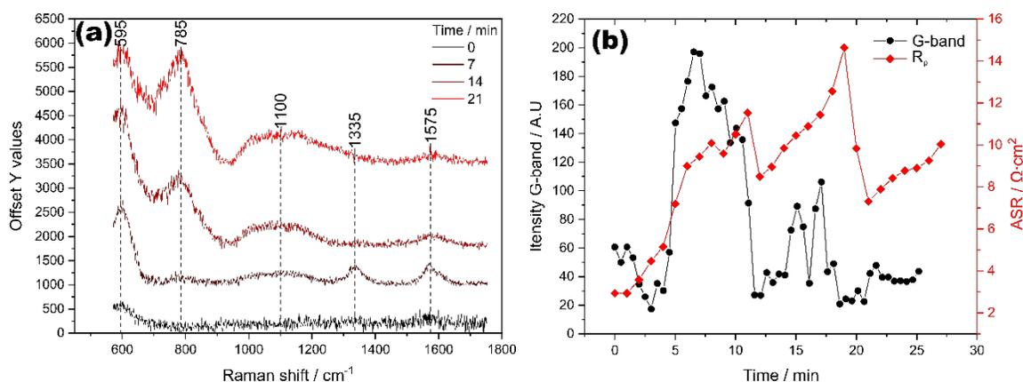
Figure 6. a) Raman spectra of the Ni-CGO infiltrated cells, when exposed to CH<sub>4</sub>, please notice that the spectra are vertically shifted for clarity and the broad peak observed around 785 cm<sup>-1</sup> originates from the STN electrode material. b) The peak intensity of the G-band plotted together with the total ASR of the Ni-CGO infiltrated cell as a function of time.
