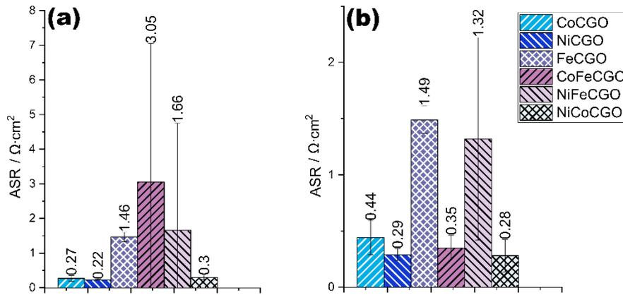
Figure 3. Averaged total ASR of the different infiltrations, in a) 4% H<sub>2</sub>O/H<sub>2</sub> at 750°C and in b) 50% H<sub>2</sub>O/H<sub>2</sub> at 750°C.
