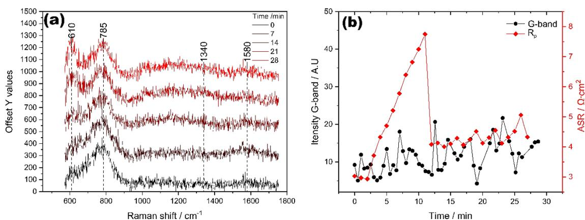
Figure 7. a) Raman spectra of the Ni-Co-CGO infiltrated cells, when exposed to CH<sub>4</sub>, please notice that the spectra are vertically shifted for clarity and the broad peak observed around 785 cm<sup>-1</sup> originates from the STN electrode material. b) The peak intensity of the G-band plotted together with the total ASR of the Ni-Co-CGO infiltrated cell as a function of time.
