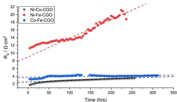
Figure 5: The total ASR as a function of time for a Ni-Co-CGO, a Ni-Fe-CGO and a Co-Fe-CGO infiltrated cell in 50% H<sub>2</sub>O/H<sub>2</sub> at 650 °C
