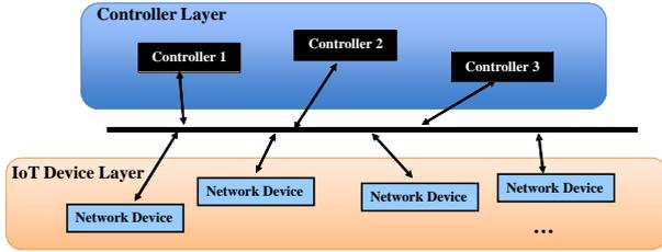
Figure 8: The high-level architecture of blockchain-based SDN.
