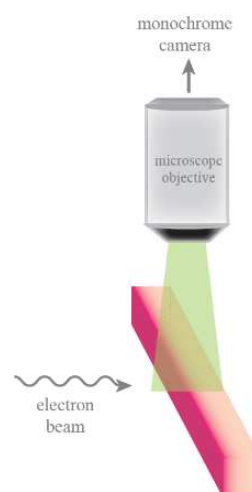
Fig.4. Simplified scheme of the readout process
