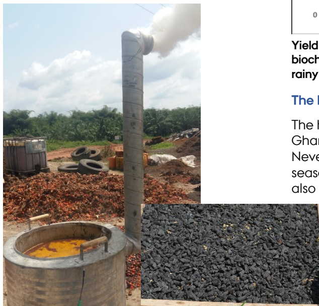
Biochar is a pyrolysis product from organic material just like charcoal. Empty fruit bunch was pyrolysed in the WEBSOC stove and the heat used for artisanal palm-oil refining
