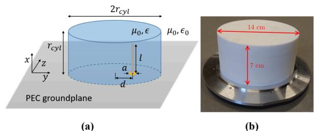
Fig. 1. (a) Sketch of the antenna, and (b) photograph of the antenna prototype.
