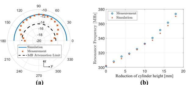
Fig. 3. (a) Simulated and measured radiation pattern ( $S_{21}$  in logarithmic scale) in the  $xy$ -plane. (b) Resonance frequency as a function of reduction of the cylinder height due to extraction of water.
