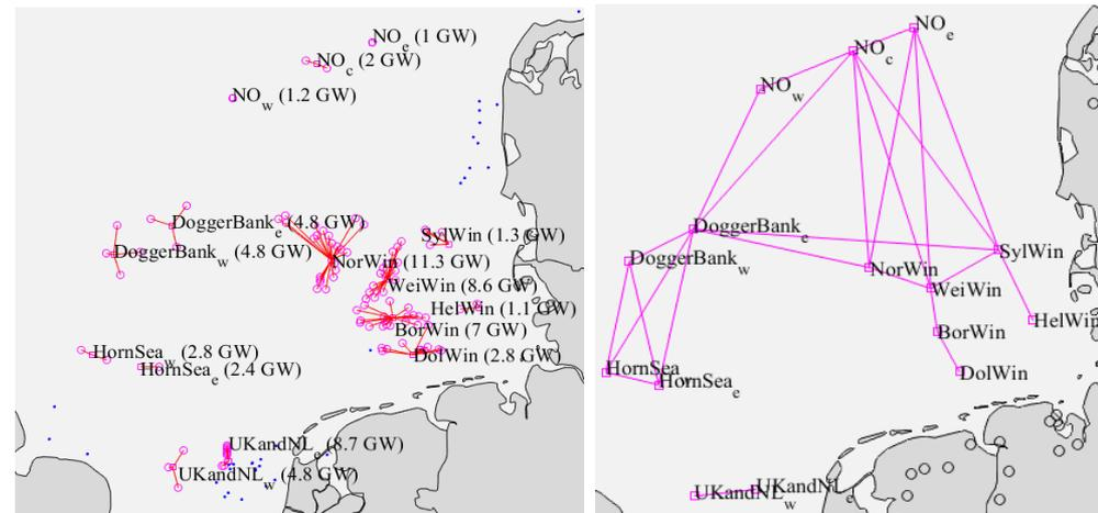
Possible hub-connected OWPP investments, and some example connections in the meshed scenario
