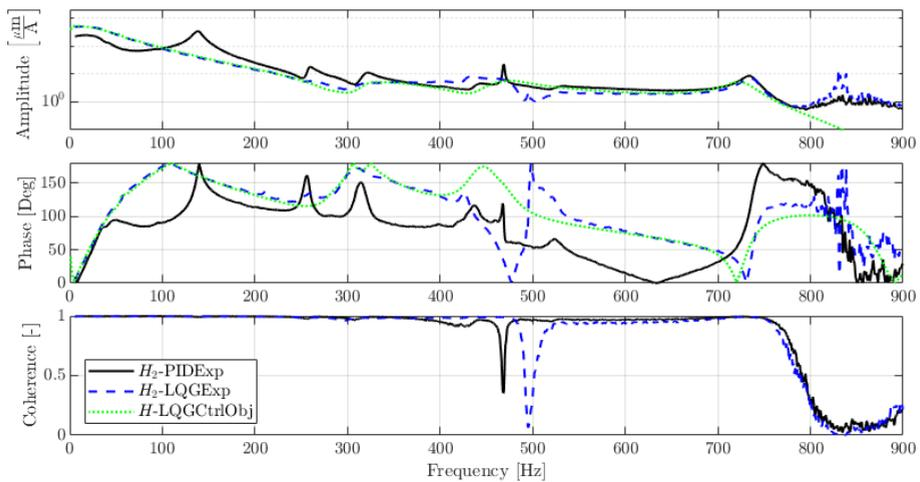
**Figure 4: Experimentally obtained frequency response for PID control design versus the experimentally obtained frequency response for LQG control design and estimated frequency response for the control object.**
