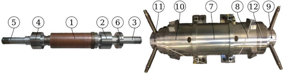
**Figure 1: Presentation of high-speed blower test facility components with included features. The shaft has a copper sheet, ①, a pair of rotor laminate stacks, ② and ④, aluminium surfaces for sensors, ③ and ⑤, and a disc with passive magnets, ⑥. The housing consists of an induction motor, ⑦, a pair of radial AMB stator geometries, ⑧ and ⑩, eddy current sensor fitting modules, ⑨ and ⑪, and axial PMB, ⑫.**
