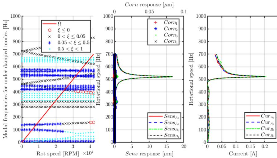
**Figure 5: Expected Campbell diagram and unbalance response for high-speed blower using PID control scheme (Centre bottom: Rotor responses; Centre top: Foundation corner responses; Right bottom: Current in coils).**
