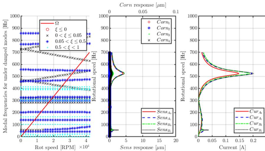
**Figure 6: Expected Campbell diagram and unbalance response for high-speed blower using LQG control scheme (Centre bottom: Rotor responses; Centre top: Foundation corner responses; Right bottom: Current in coils).**
