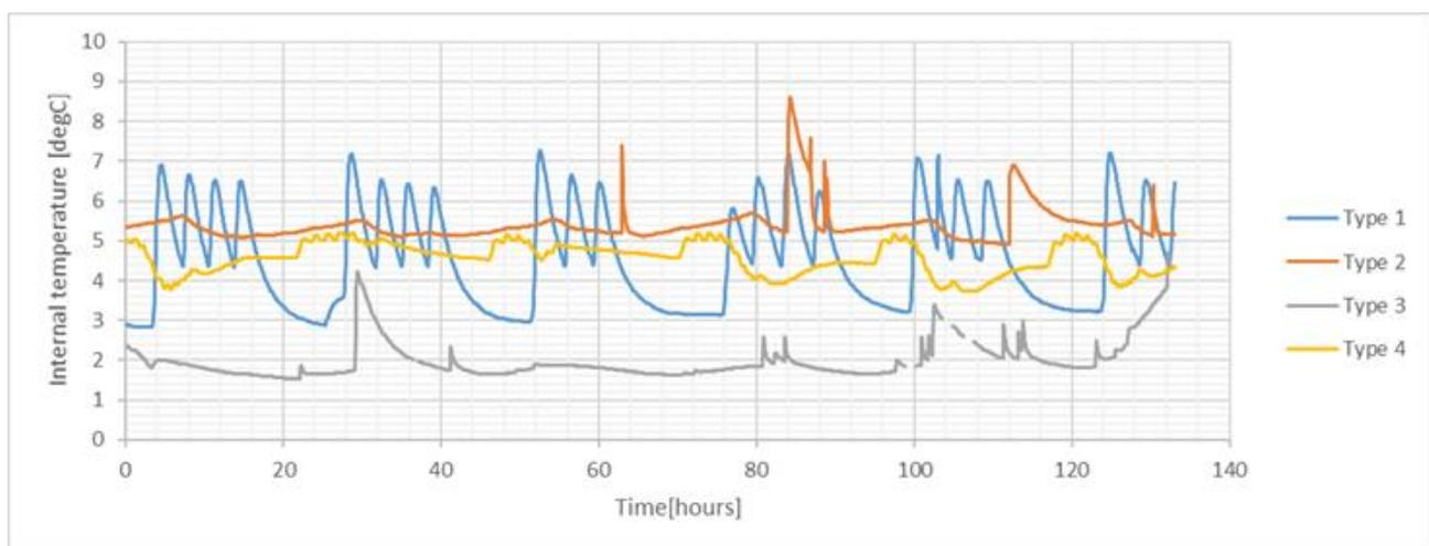
**Figure 4: Example of field test data (from four different sites). This figure represents four different models of vaccine coolers in the ongoing SolarChill project. Every type of refrigerator has its own temperature “fingerprint” that may be useful in preventive maintenance.**
