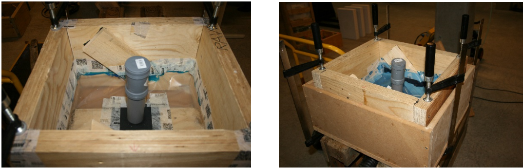
Figure 3. Test equipment for test of airtightness. Left: wooden frame with lining of membrane taped to the frame, pipe with collar in the middle. Right: wooden frame placed in box, a ventilator created a pressure difference between frame and box through a hole in the box (not visible on photo).
