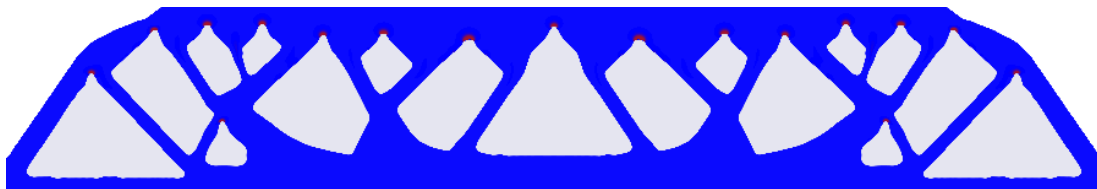
Figure 8: The optimized result with zero Neumann boundaries for the PDE filter, while other optimization parameters are the same as those of Figure 7 (b). The final compliance is C = 206.08 .
