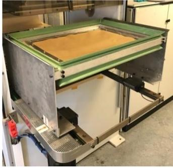
**Figure 1.** Carrier to transport material between the two sections of the press consolidation facility.
