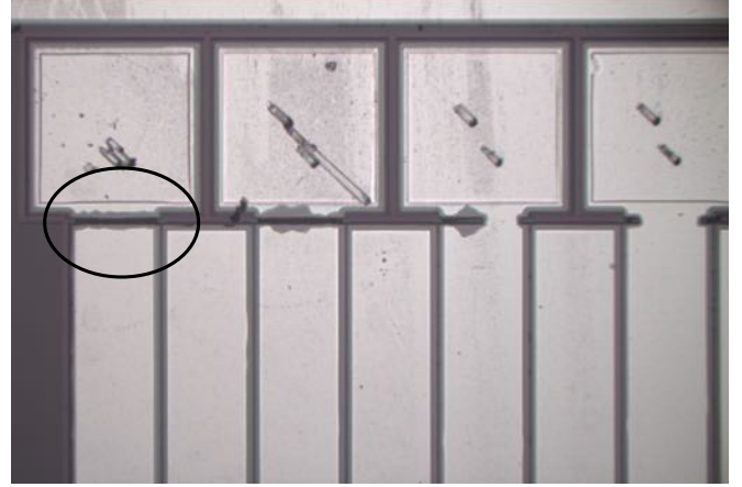
Fig. 6. Bond pad and row element not connected due to errors in the lithographic process.
