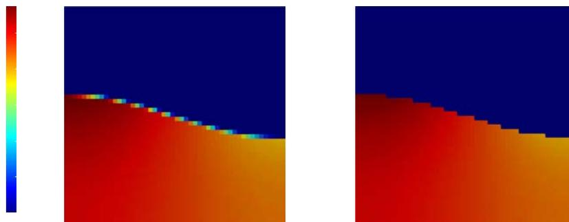
The currently freely available Volume Of Fluid model in the open source software OpenFOAM does not capture the behavior of the pressure correctly close to the free surface. The density jumps at the surface, which can be illustrated by examining the dynamic pressure.
