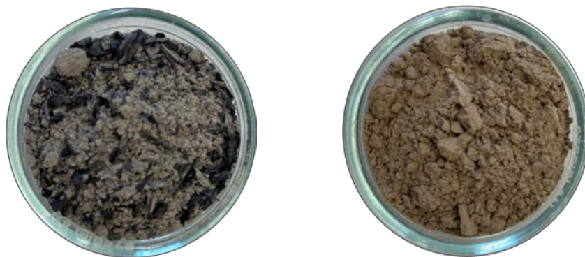
Figure 13. WA1 (left) and WA2 (right) as received. Diameter of petri dishes = 40 mm.
