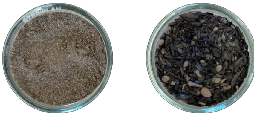
Figure 14. WA1 < 250 \mu m (left) and WA1 > 250 \mu m (right). Diameter of petri dishes = 40 mm.
