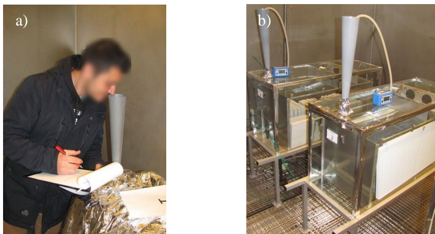
Figure 2.4 a) Subject sniffing and a glass chamber covered with aluminium foil. b) Sampling by Tenax TA tube.
