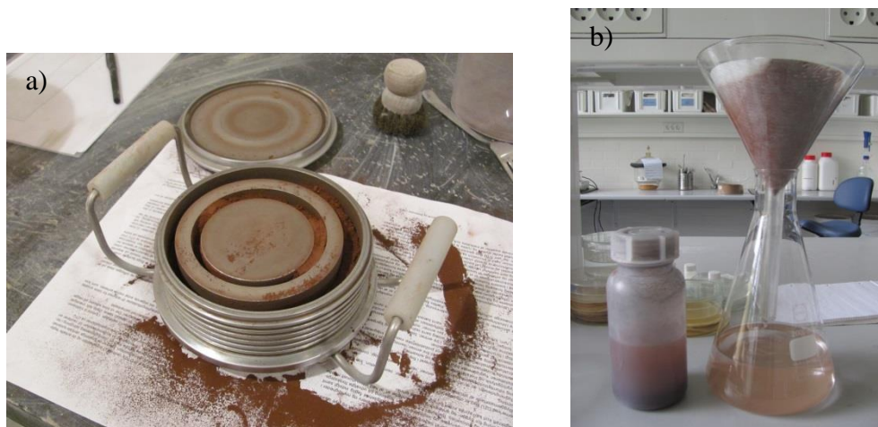
Figure 2.2 a) Ash grinding; ash placed in a cup with grinding rings b) Water washing of ash
