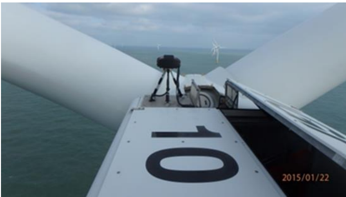
Figure 19 Picture of the Wind Iris on the nacelle of turbine IGF10.
