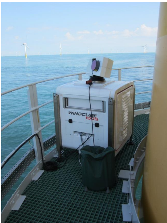
Figure 11 Picture of WINDCUBE 100S after commissioning on the turbine transition piece platform. The scanning head of the lidar (middle of the window) was at 1.3m above the top of the transition piece railing.
