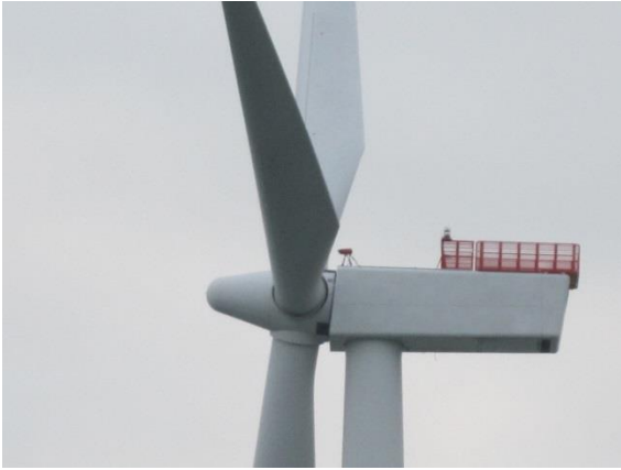
Figure 18 Picture of the Wind Iris on the nacelle of turbine IGF10. The front of the optical head was 0.5m behind the rotor.
