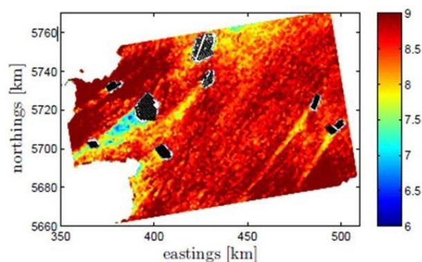
Wind farm wakes observed by satellite radar in Belgium and UK North Sea. The black colour indicates wind farms. Lower winds southwest of each wind farm are the wake (lee effect). The wind is blowing from the northeast. Wind speed in m/s. Source: DTU Wind Energy.
