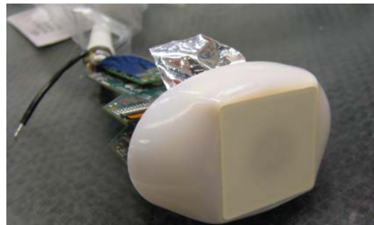
Fig. 4. The nose piece connected to the electronics after the outer lens had cured. The metal sheet sticking out of the nose piece is the electromagnetic shield.
