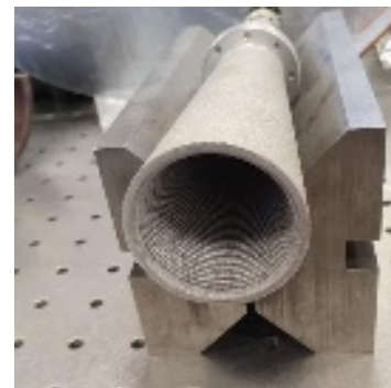
FIG. 2. Aluminum horn made by additive manufacturing.
