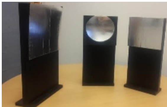
FIG. 1. Quasi-optical mirrors produced by FDM and aluminum foil.
