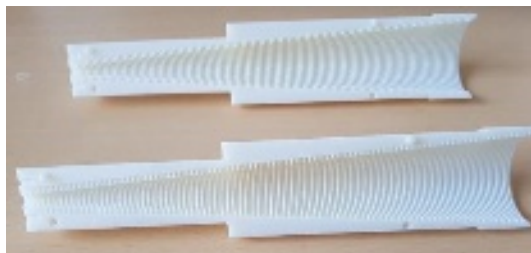
FIG. 3. 60 GHz corrugated horn 3D plastic printed in a FORTUS 5 450mc FDM printer.
