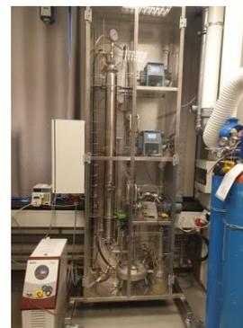
The obtained results from the laboratory scale experiments are currently being confirmed in a pilot scale TBR under the respective operational conditions. Syngas from a gasifier is also being tested in the pilot scale TBR.
