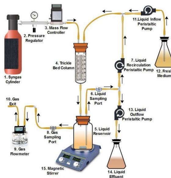
Figure 1. Process Flow Diagram of the lab scale bioreactor configuration [2]
