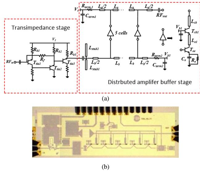
Fig. 2. (a) Simplified circuit diagram of the amplifier subsystem. (b) Chip photo ( $1.8 \times 1 \text{ mm}^2$ ).
