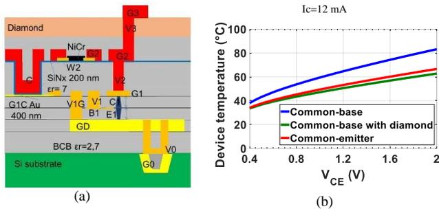
Fig. 1(a). Layer stack of the transferred-substrate process. (b) Self-heating improvement of common-base transistor ( $0.5 \times 5 \mu\text{m}^2$ ) using diamond heat spreader.
