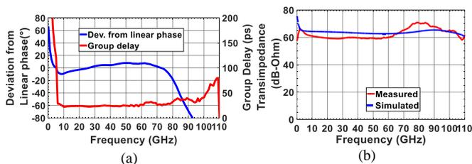
Fig. 4. (a) Group delay (ps) and deviation from linear phase (°) vs frequency and (b) transimpedance (Z<sub>21</sub>) in dB-Ω vs. frequency (GHz)
