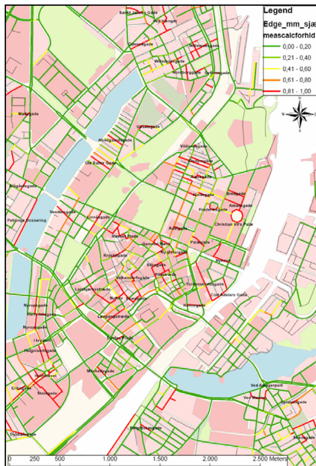
Figure 10: Signal fallouts scale per road in Copenhagen (road map based on KRAKS kdv geodatabase, www.krak.dk )
