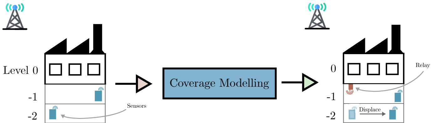
Fig. 1: Indoor deployment situations are further complicated by deep-indoor situations such as basements where coverage modelling is difficult and impractical. Current models perform well at indoor deployment situated at level 0 and above but are inaccurate at level -1 and -2. This paper presents measurements conducted at level -1 and -2.
