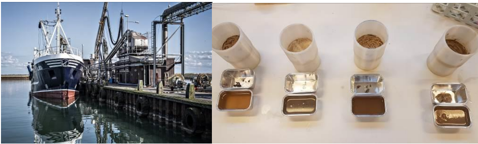
Figure 2: Landing of fish at TripleNine at Thyborøn (left) and evaluation flocculant efficiency and dosage using MC Higgins' test (right).
