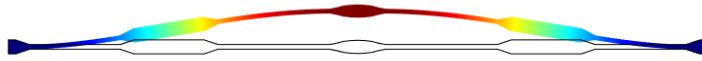
Fig. 3. The fundamental flexural mode the new design for maximizing the hardening behavior of a clamped-clamped beam. The color denotes the total displacement. The mode shape is obtained by using COMSOL Multiphysics 5.4 with 2D solid element.
