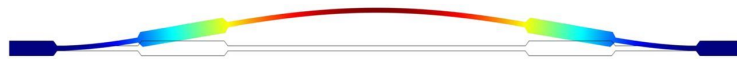
Fig. 4. The fundamental flexural mode of the design in [14] for maximizing the hardening behavior of a clamped-clamped beam. The color denotes the total displacement. The mode shape is obtained by using COMSOL Multiphysics 5.4 with 2D solid element. The image is re-used from [14].
