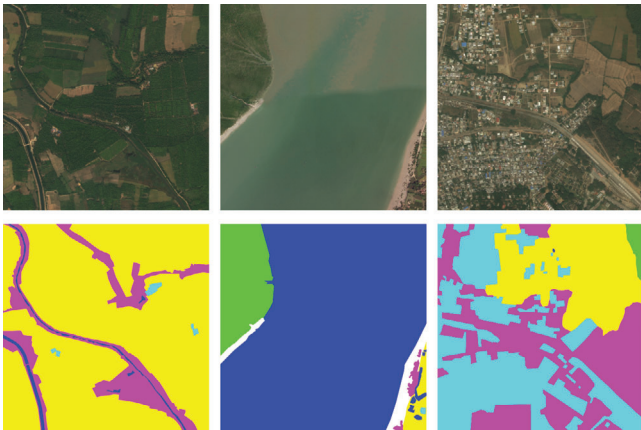
Fig. 2 First row: original images used for training and validation. Second row: the corresponding mask. See Table 1 for colour encoding
