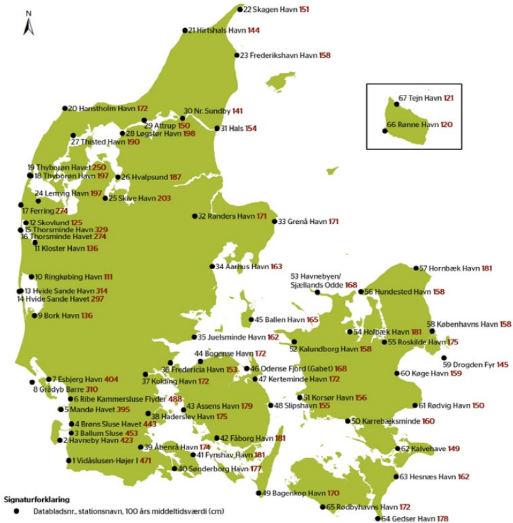
Figure 2: Placement of the 67 gauge stations in Denmark. The red values next to the station name indicates the water level causing a 100-year flood event. Source: (Kystdirektoratet, 2019).
