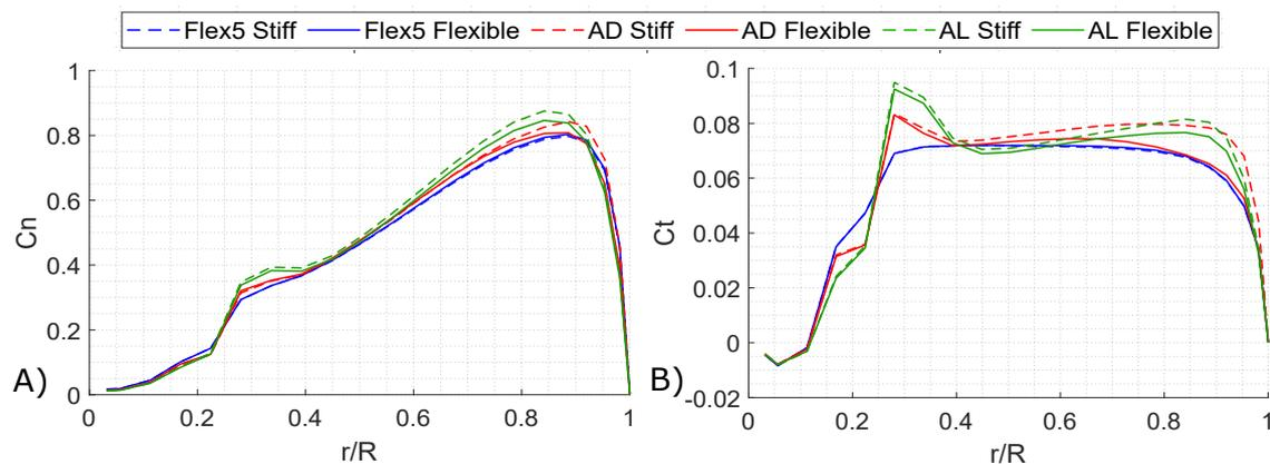
**Figure 5.** Normalised mean blade loads,  $U = 10$  m/s: A) normal; B) tangential
