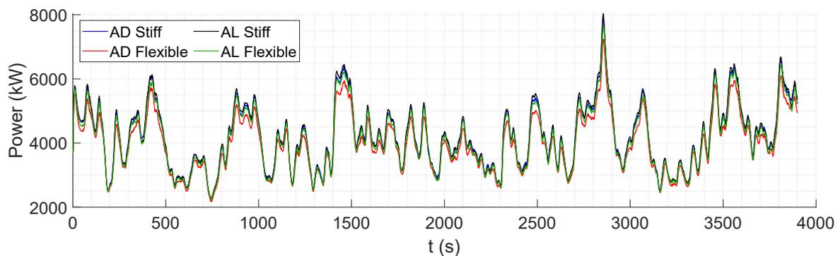
**Figure 6.** Power output against time for 8m/s
