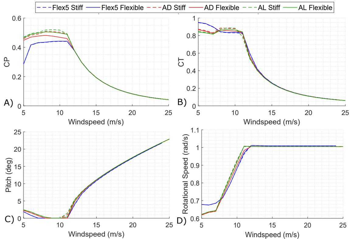
**Figure 4.** Steady state performance: A) Power coefficient CP; B) Thrust coefficient CT; C) Pitch angle; D) Rotational Speed
