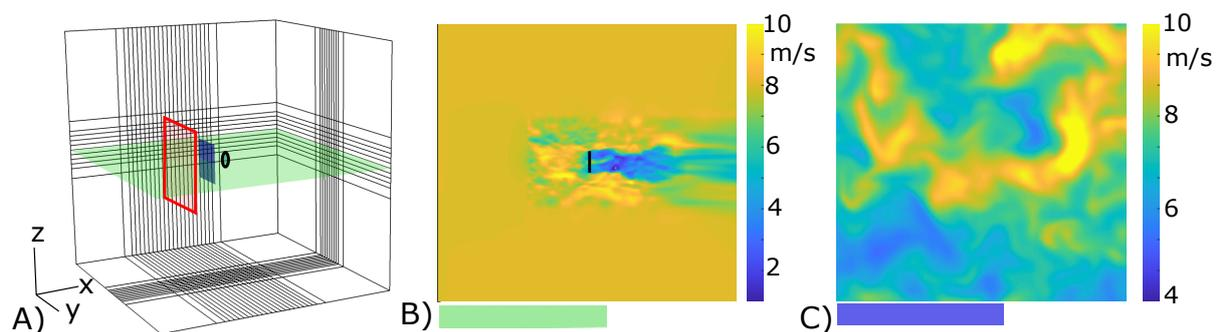
**Figure 1.** Domain setup: A) domain (every 8th line shown for clarity), red square shows turbulent body forces application, black circle shows turbine position; B) velocity magnitude over green plane for AD simulation; C) velocity magnitude over blue plane.
