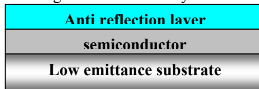
Fig-2 schematic diagram of semiconductor/Metal tandems as an selective absorber
