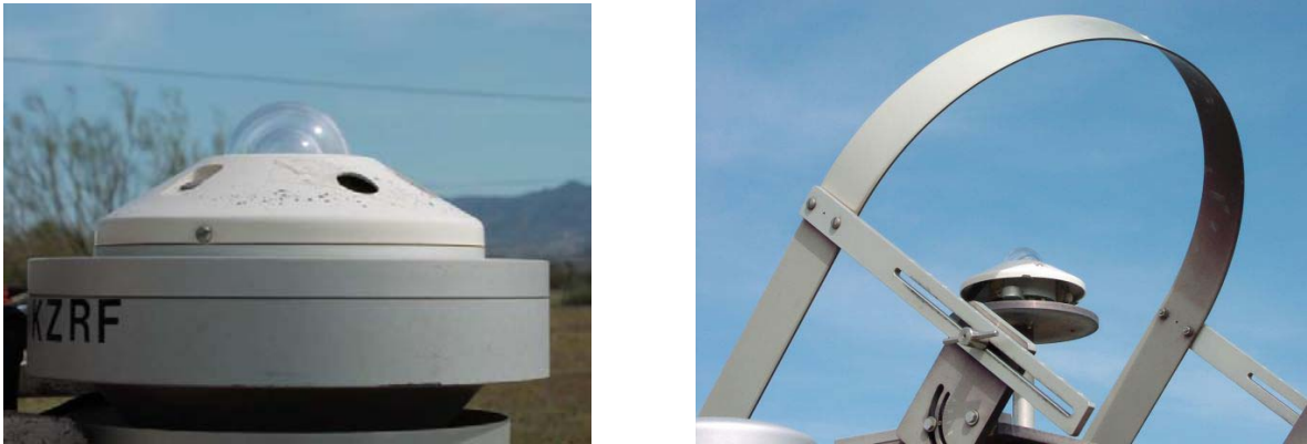
Figure 4: Pyranometers used for measuring the global radiation (left) and diffuse radiation (right).
