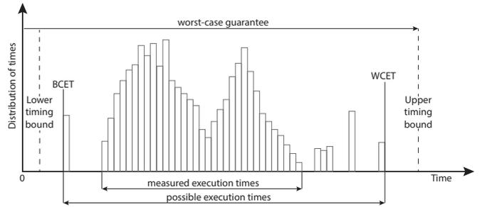
Fig. 2. Basic notions of timing analysis [7].
